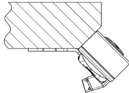
**To mount the panel:** Just click the panel into the bracket and it is fixed.
