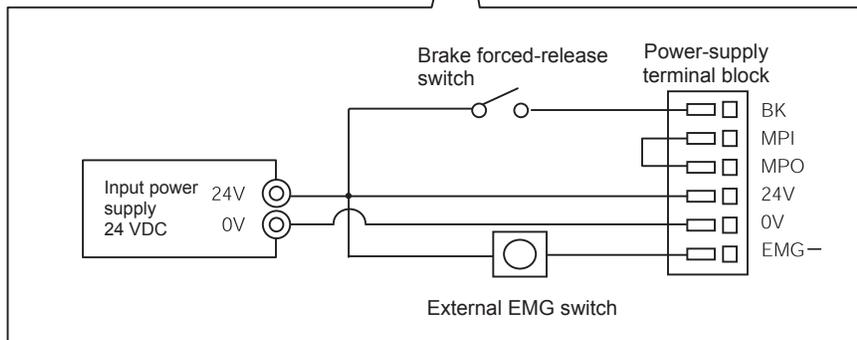
**Caution:** The BK terminal need not be connected if the actuator has no brake.
