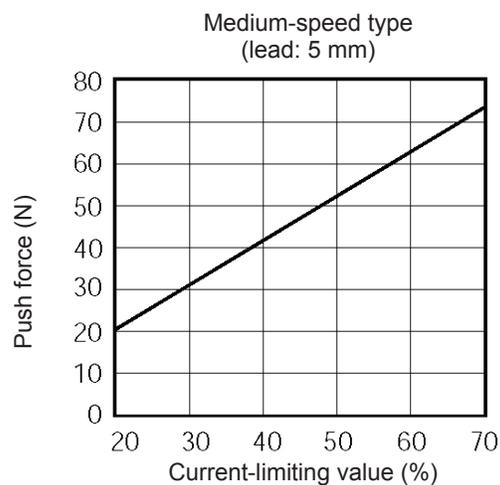
**Caution:** Accuracy of push force while the actuator is standing still is not guaranteed. The above figures should be used for reference purposes only. Take note that if the push force is too small, the actuator may malfunction during push-motion operation due to slide resistance, etc. The maximum current-limiting values are as shown in the graphs above. The minimum current-limiting values should be at least 20%.
