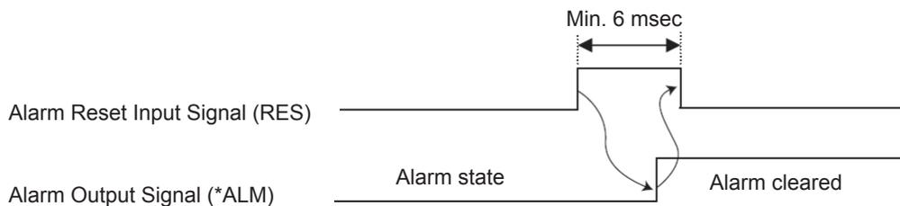
**Note:** Whatever the alarm, always investigate the cause of the alarm and remove the cause before resetting the alarm. If the cause of the alarm cannot be removed, or when the alarm cannot be reset even after the cause has been removed, please contact IAI.
