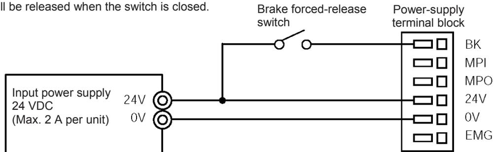
**Danger:** If the actuator is oriented vertically, exercise due caution when releasing the brake to prevent the slider/rod from dropping unexpectedly to pinch your hand or damage the robot hand or work.
