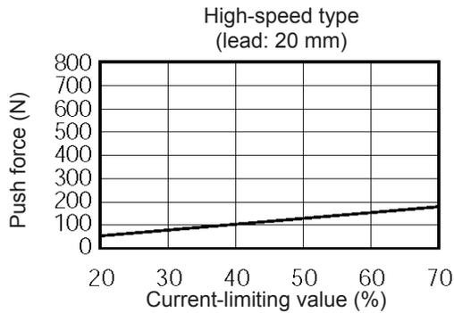
**⚠ Caution:** Accuracy of push force while the actuator is standing still is not guaranteed. The above figures should be used for reference purposes only. Take note that if the push force is too small, the actuator may malfunction during push-motion operation due to slide resistance, etc. The maximum current-limiting values are as shown in the graphs above. The minimum current-limiting values should be at least 20%.
