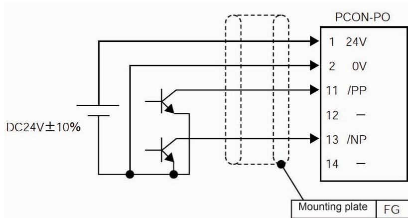
Note 1 Always connect the shield of the twisted pair cable joined to the connector, to the mounting plate.
