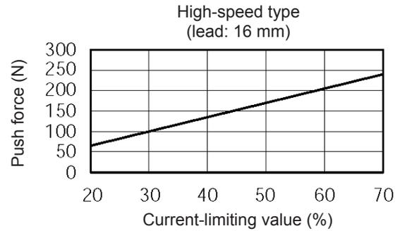
**⚠ Caution:** Accuracy of push force while the actuator is standing still is not guaranteed. The above figures should be used for reference purposes only. Take note that if the push force is too small, the actuator may malfunction during push-motion operation due to slide resistance, etc. The maximum current-limiting values are as shown in the graphs above. The minimum current-limiting values should be at least 20%.
