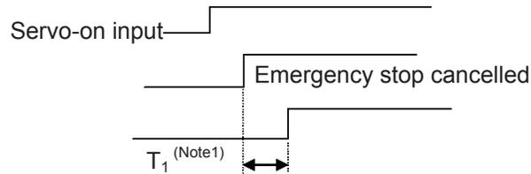
(Note 1)  $T_1$ : Excited-pole detection time = 0.2 to 12 sec
