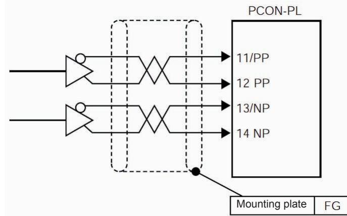
Note Always connect the shield of the twisted pair cable joined to the connector, to the mounting plate.
