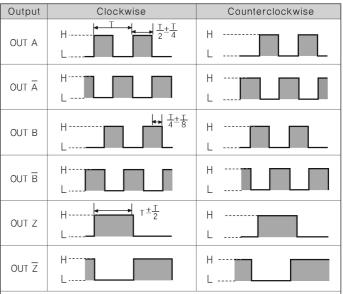
Clockwise (CW): When you are looking at the shaft of the product, it is turning in a clockwise direction. Counterclockwise (CCW): When you are looking at the shaft of the product, it is turning in a counterclockwise.
