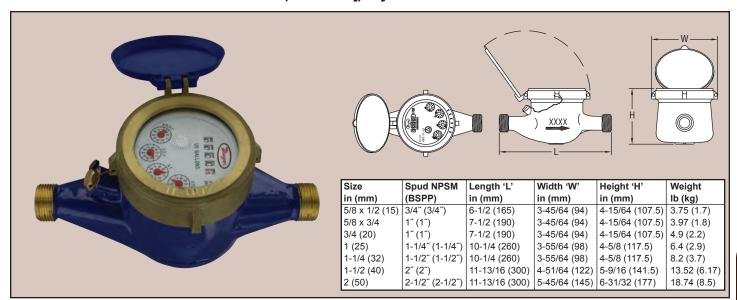
The Series WM2 Multi-Jet Water Meter is ideal for commercial and industrial applications. The multi-jet design allows for simplicity and accuracy with wide flow ranges, even in low flow applications. The magnetically driven, hermetically sealed register will not leak or fog and is completely separated from the water. These water meters are designed for long service life and maintenance-free operation, even under harsh conditions.
