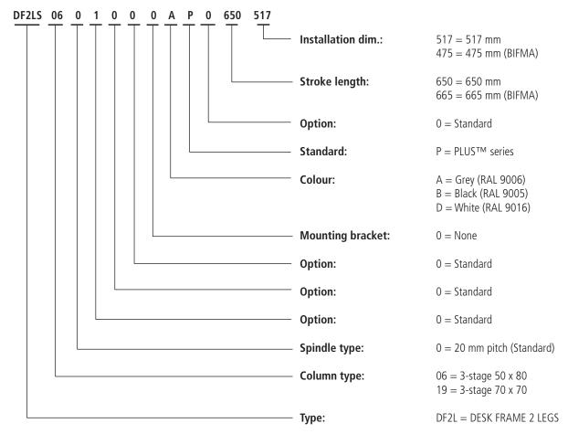
The installation dimensions of the column (517/475 mm) plus the beam correspond to installation dimensions of our standard columns (560/518 mm).
