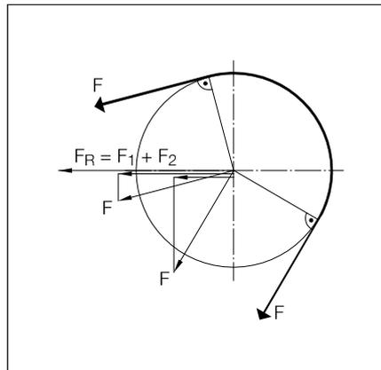
For measuring purposes, only those components, i.e.  $F_1$  and  $F_2$  effective in the direction of measuring, are relevant. The resultant measuring force is the sum of  $F_1 + F_2$ . This is halved, given centred web travel, between the two load cells.
