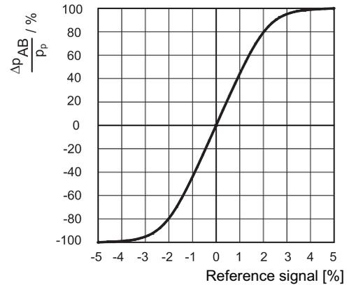
The diagram shows the valve pressure gain, expressed as % of the ratio between the port pressure variation in A or B ( $\Delta p_{AB}$ ) and the P system pressure, according to the reference signal.
