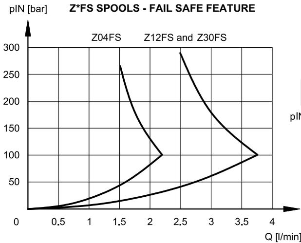
Flow P→B / A→T with valve in fail safe position, depending on the incoming pressure.
