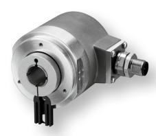
Absolute multiturn encoders detect any angle within a full revolution of 360° and also the number of revolutions. With absolute encoders, each incremental angle is assigned a code pattern. This allows the position to be detected at any time, even after a power failure, without having to initialize a reference run. Absolute encoders detect angles, positions and inclinations precisely – tasks, that are typically found in robotics, positioning and process technology.
