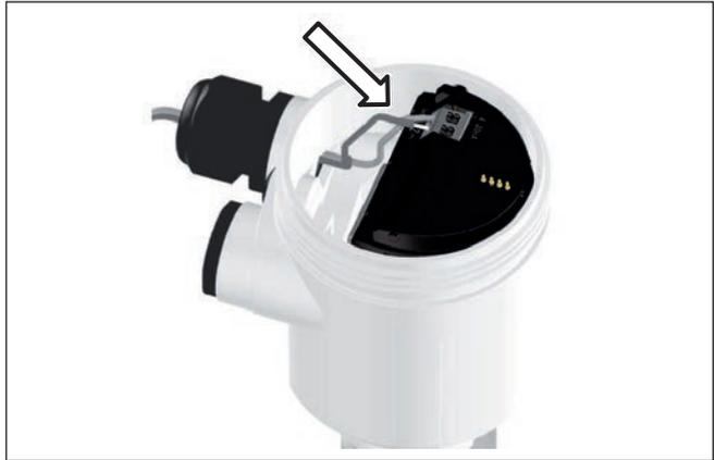
Fig. 20: Connection steps 5 and 6 - Single chamber housing
