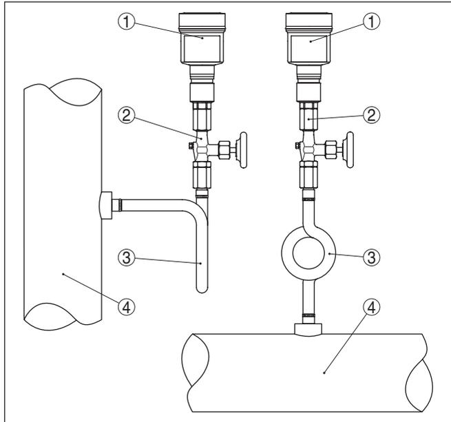
Fig. 16: Measurement setup with process pressure measurement of gases in pipelines
