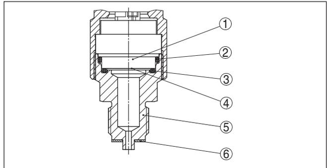
Fig. 4: Recessed installation of the measuring cell (example: manometer connection G½)
