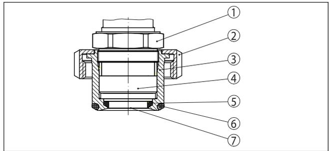
Fig. 36: VEGABAR 82, structure of the hygienic connection with compression nut
