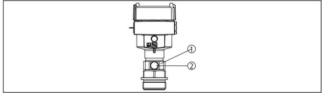
Fig. 12: Position of the filter element - Ex-d version
