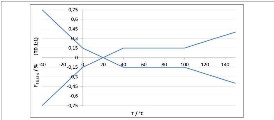
Fig. 39: Basic temperature error  $F_{TBasis}$  at TD 1 : 1
