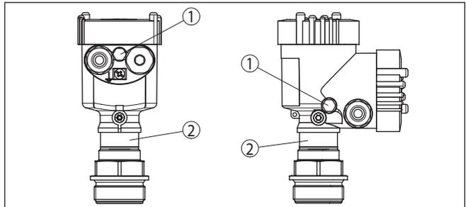
Fig. 13: Position of the filter element - gastight leadthrough
