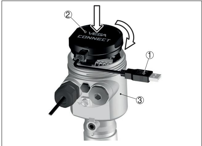
Fig. 34: Connection of the PC directly to the sensor via the interface adapter
