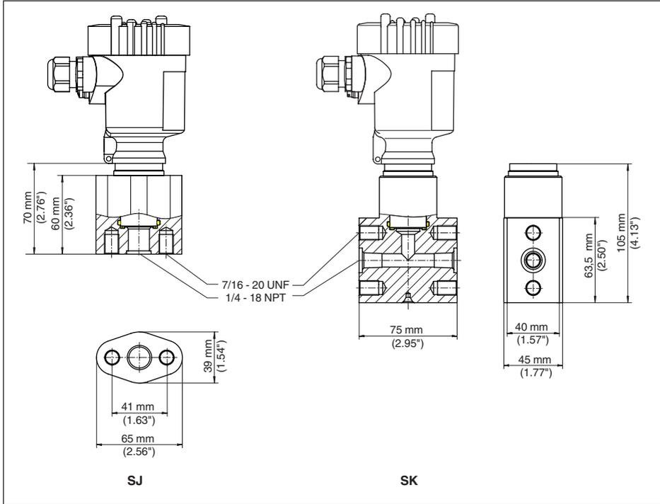
Fig. 52: VEGABAR 82, connection acc. to IEC 61518
