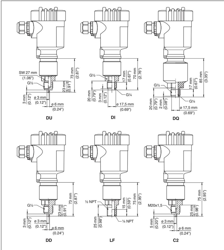
Fig. 46: VEGABAR 82, threaded fitting not front-flush
