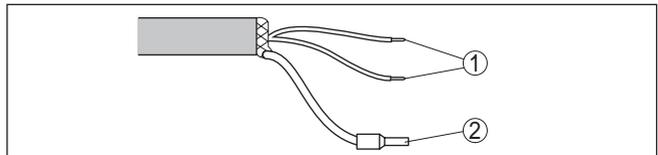
Fig. 25: Wire assignment in permanently connected connection cable
