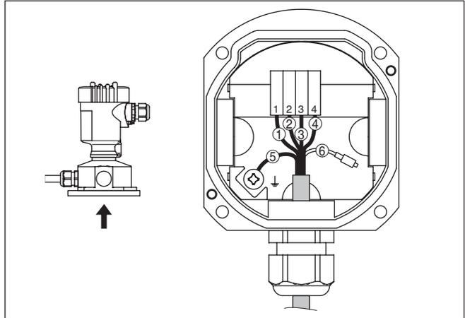
Fig. 28: Connection of the sensor in the housing base
