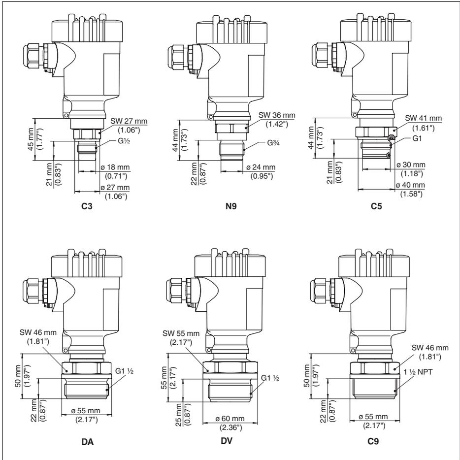
Fig. 47: VEGABAR 82, threaded fitting front-flush
