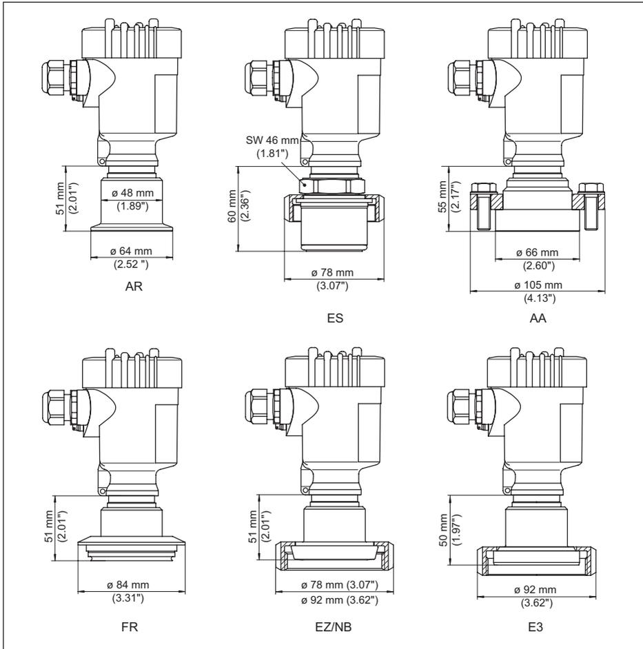
Fig. 48: VEGABAR 82, hygienic fitting
