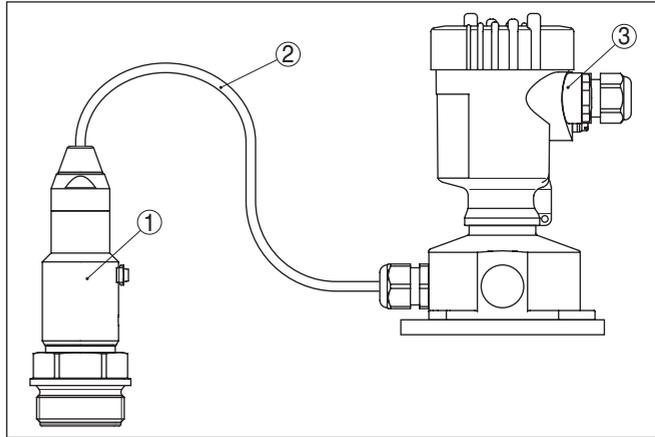
Fig. 26: VEGABAR 82 in IP 68 version 25 bar with axial cable outlet, external housing
