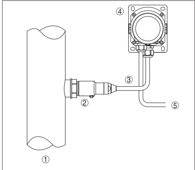
Fig. 19: Configuration, process module, external housing
