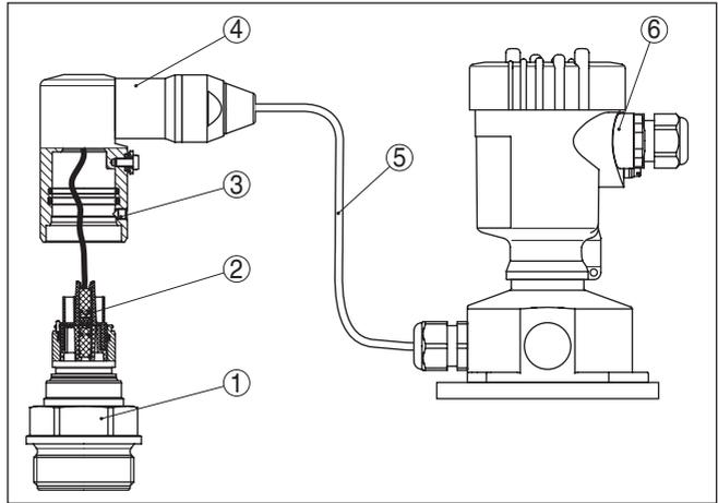
Fig. 37: VEGABAR 82 in IP 68 version, 25 bar and lateral cable outlet, external housing
