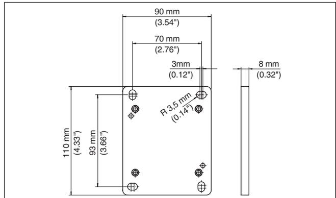
Fig. 20: Drilling template - wall mounting plate
