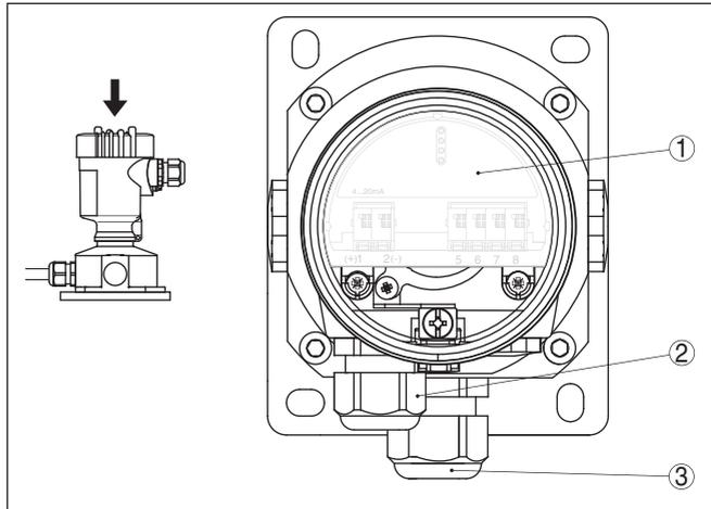
Fig. 27: Electronics and terminal compartment
