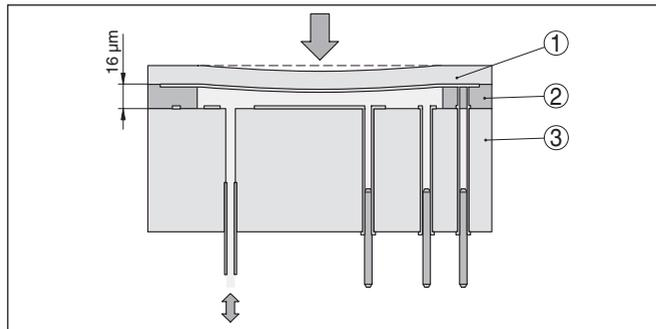
Fig. 3: Configuration of the CERTEC® measuring cell
