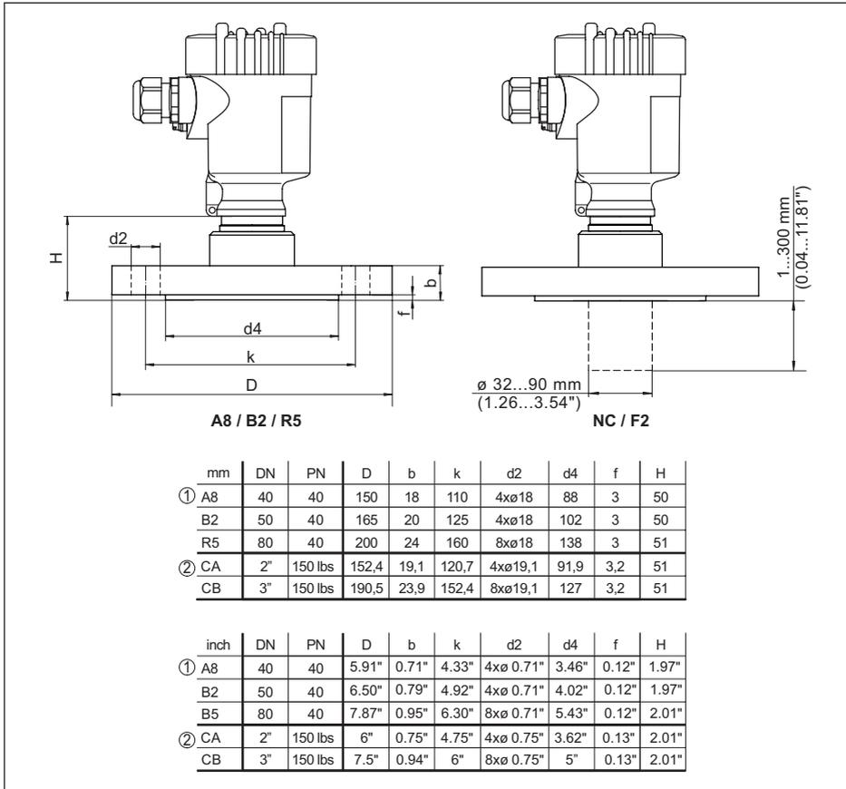
Fig. 49: VEGABAR 82, flange connection
