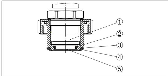
Fig. 8: Hygienic installation of the measuring cell (example: hygienic fitting with compression nut)
