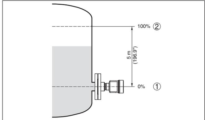
Fig. 33: Parameter adjustment example "Min./max. adjustment, level measurement"
