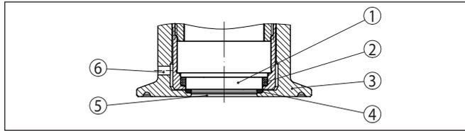
Fig. 9: Hygienic installation of the measuring cell acc. to 3-A (example: Clamp connection)
