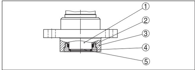
Fig. 7: Front-flush installation of the measuring cell with double seal (example: flange connection with extension)
