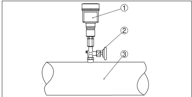
Fig. 15: Measurement setup for process pressure measurement of gases in pipelines
