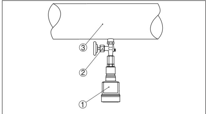
Fig. 17: Measurement setup for process pressure measurement of liquids in pipelines
