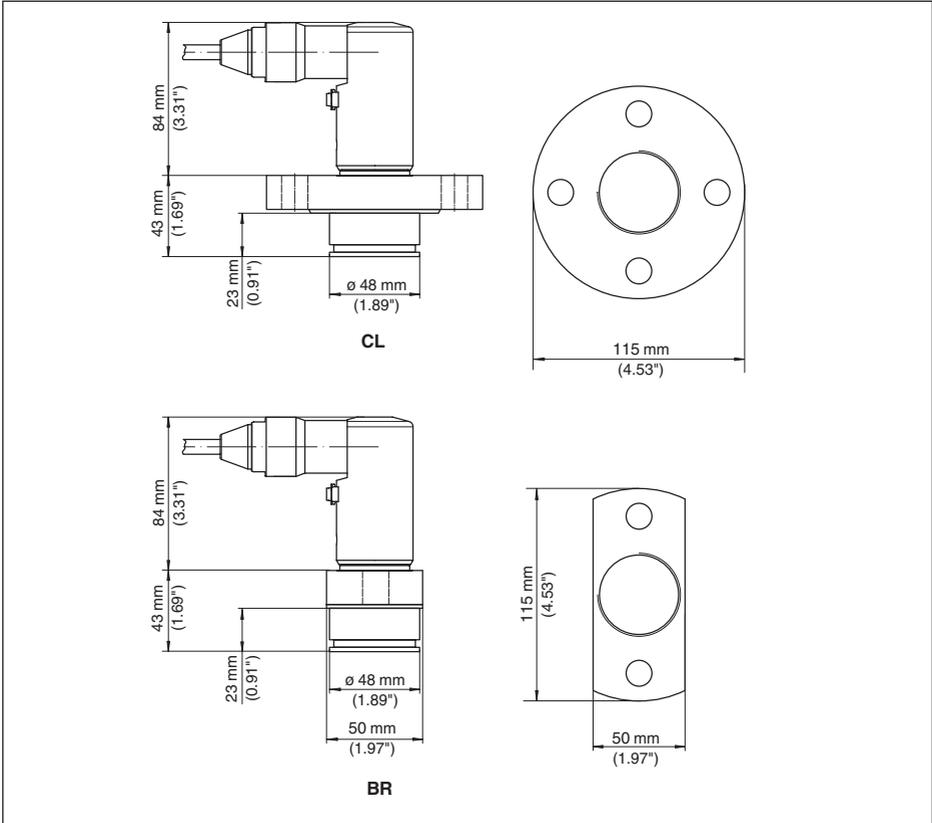
*Fig. 51: VEGABAR 82, flange connection for the paper industry: CL = absolutely front-flush for headbox, BR = absolutely front-flush for headbox (flange 2-times flattened)*
