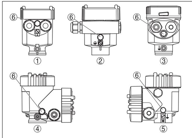
Fig. 11: Position of the filter element - non-Ex, Ex-ia and Ex-d-ia version
