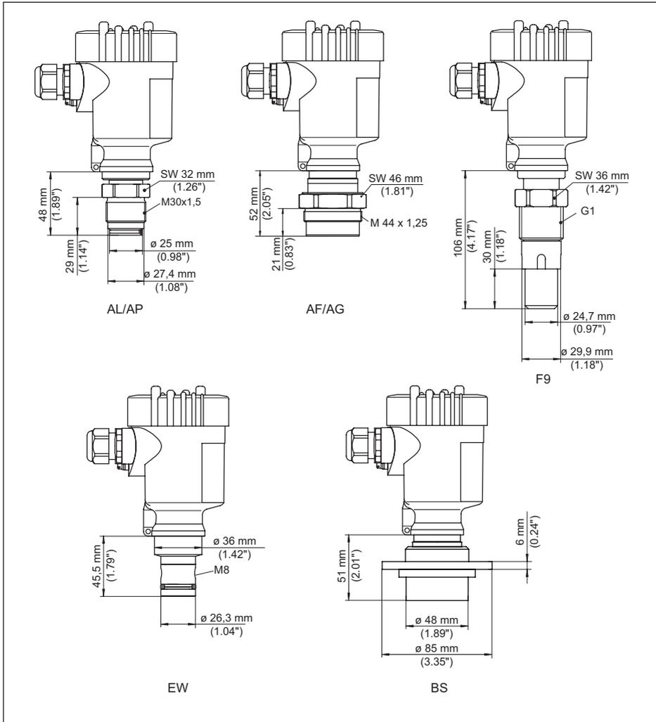
Fig. 50: VEGABAR 82, extension fitting
