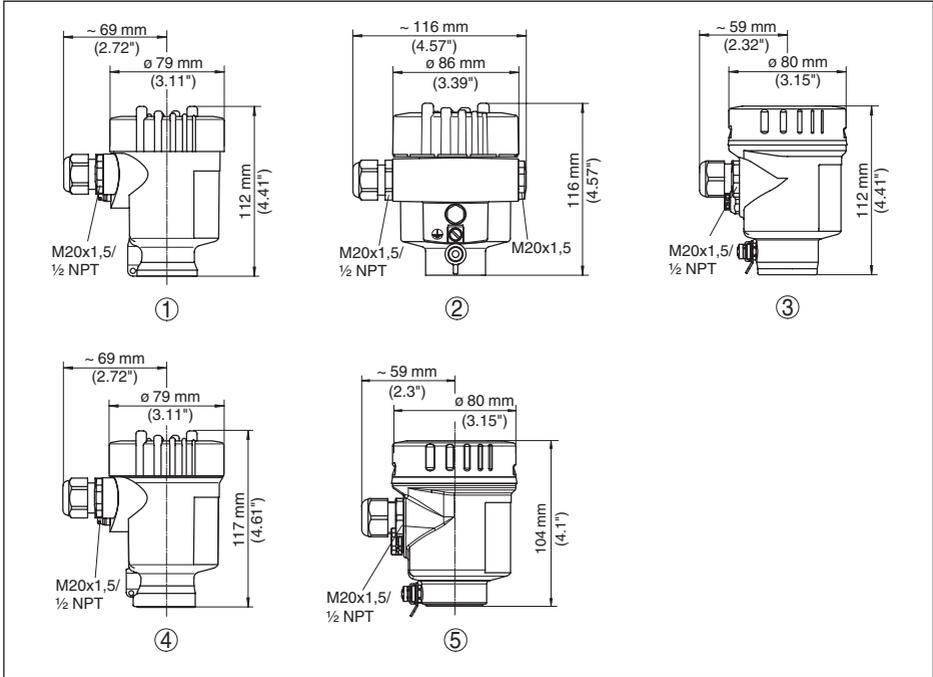
Fig. 44: Housing versions in protection IP 66/IP 67 and IP 66/IP 68 (0.2 bar)
