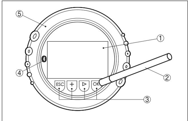
Fig. 32: Display and adjustment elements - with adjustment via magnetic pen
