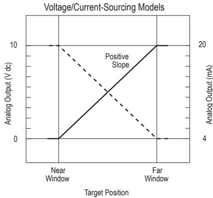
On = Direct = Output value (voltage or current) increases with increasing distance of the target from the sensor
