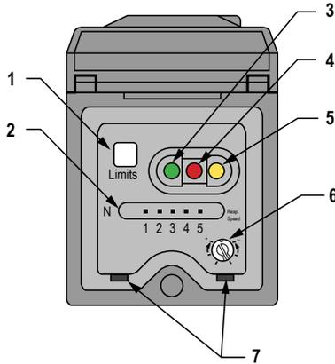
1. Button for programming the sensing window limits
