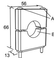
Hole center spacing: A=ø 45
