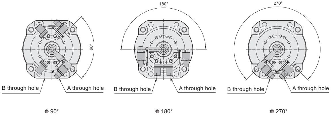
⊙ Cushion position block shows as above figure. It could be choice shock absorber for rotating position and adjust angle. The angle range will be 0 ~ -10°
