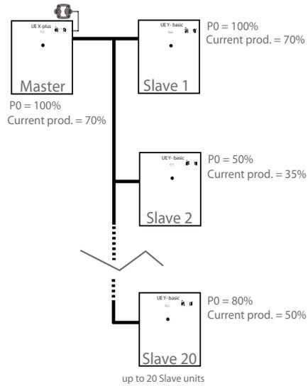
Connection between UEX Master and Slave UEY for the connect using cable shielded.
