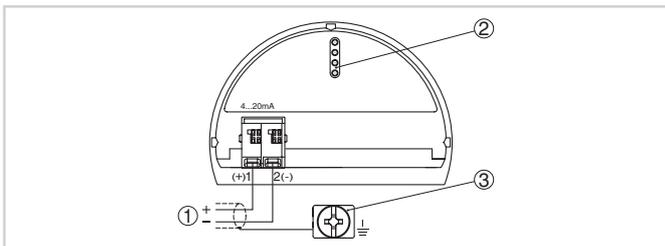
Electronics and terminal compartment, single chamber housing
