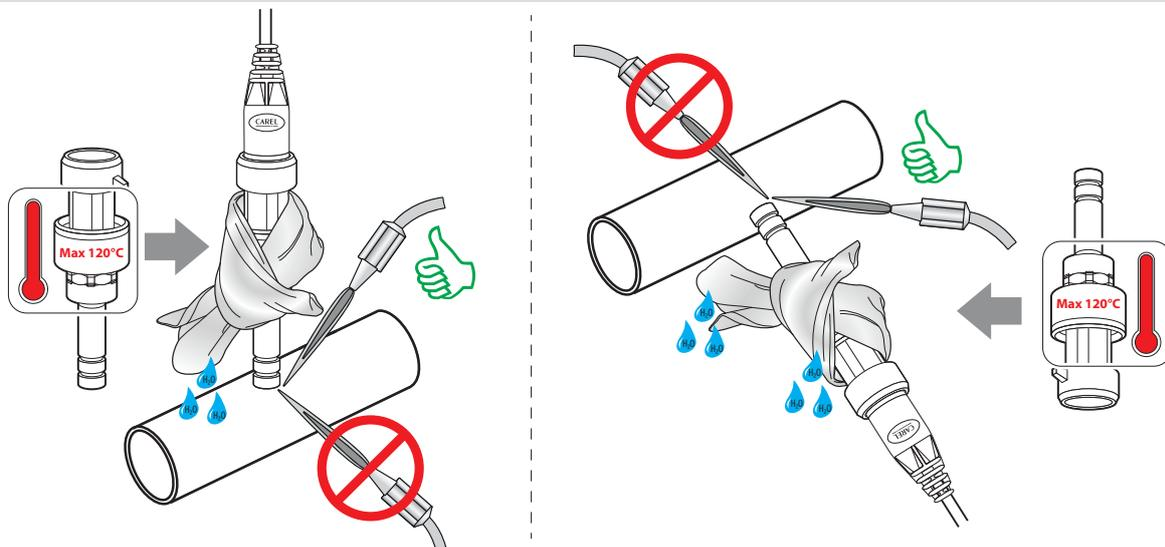
⚠️ Wrap a wet rag around the sensor body and weld without overheating the sensor, aiming the flame at the end of the pipe.
