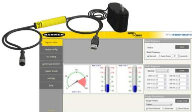
The User Configuration Tool (UCT) offers an easy way to link I/O points in your wireless network, view I/O register values graphically, and set system communication parameters when a host system is not part of the wireless network.
