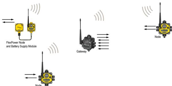
The SureCross® DX80 wireless I/O network provides reliable monitoring without wiring or conduit installation. The SureCross wireless network operates independently or in conjunction with a host system, PLC, and/or PC software.
