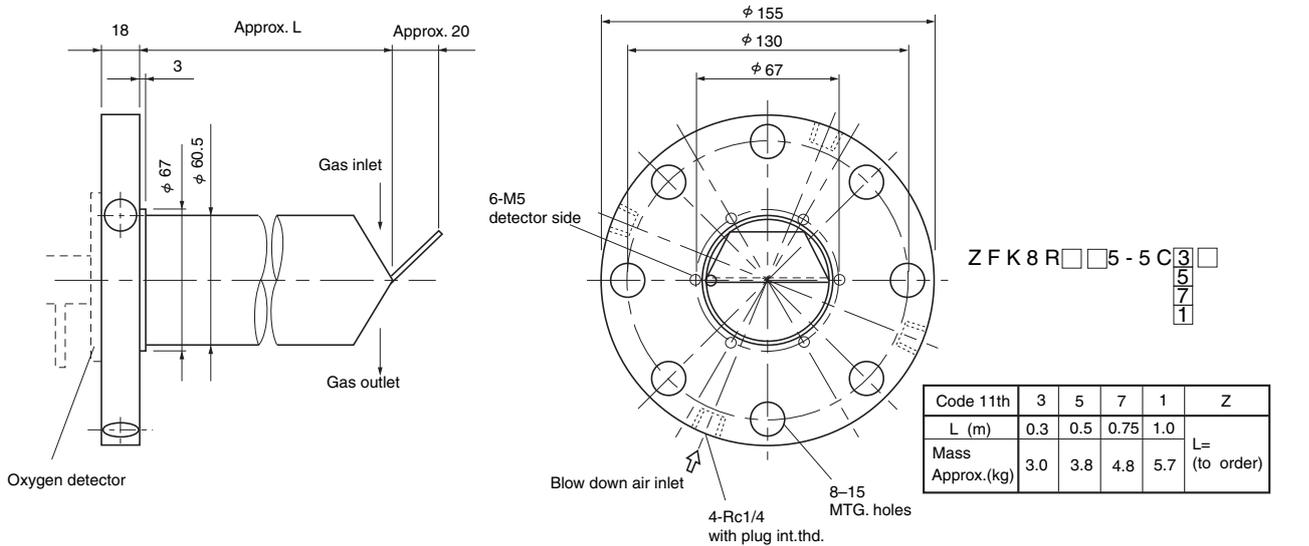
Flow guide tube (for high particulate)
