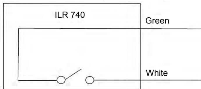
Figure 17: ILR 740 wiring
