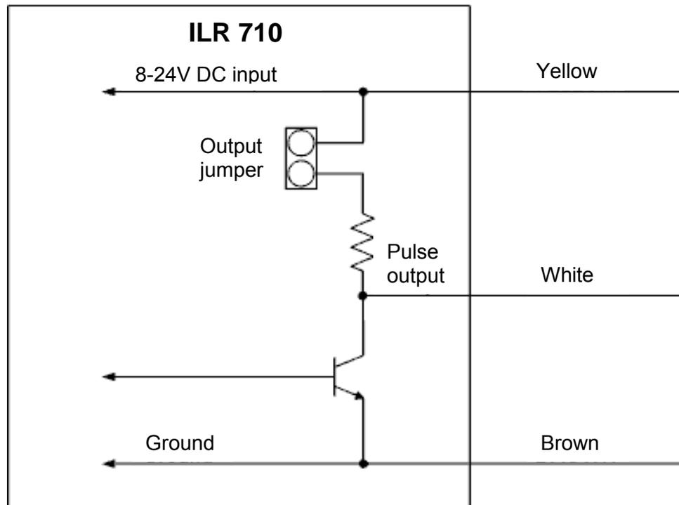
Figure 13: ILR 710 wiring
