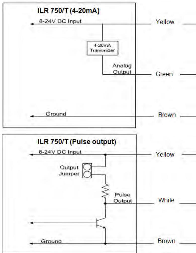
Figure 18: ILR 750 / 750T wiring
