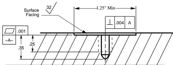
Figure 1: Stud Mounting: Surface Preparation
