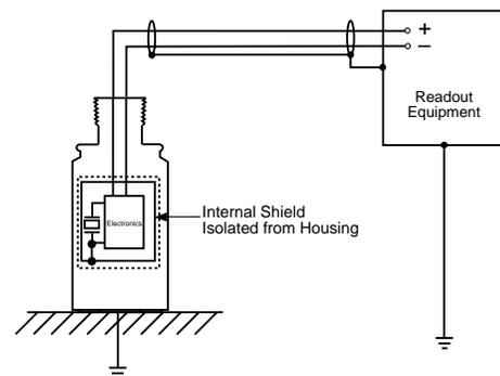
Figure 2: Multiconductor/Shield Configuration
