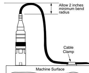
Figure 3: Cable Anchoring
