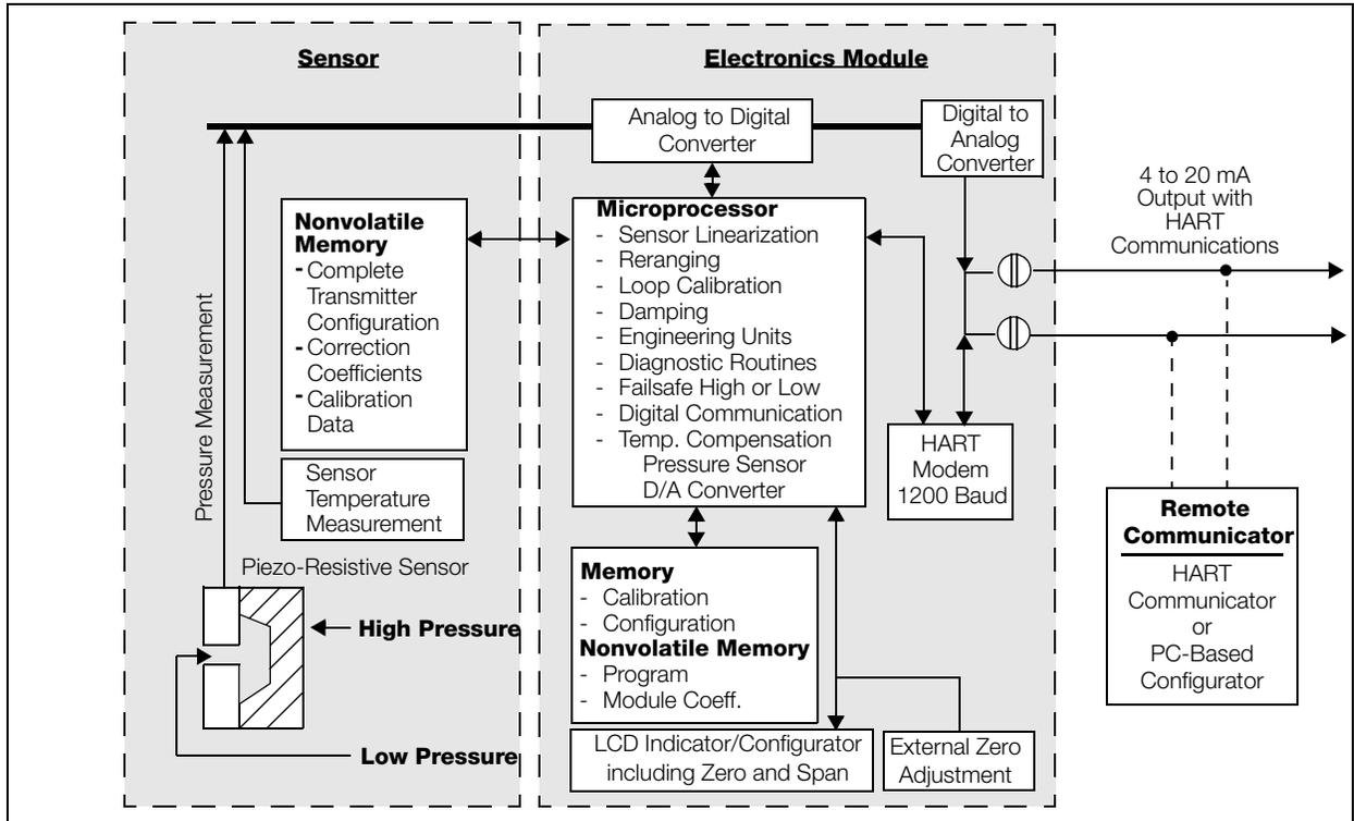
Figure 17. Transmitter Functional Block Diagram
