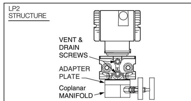
Figure 15. Adapter Mount to Existing Coplanar Manifold
