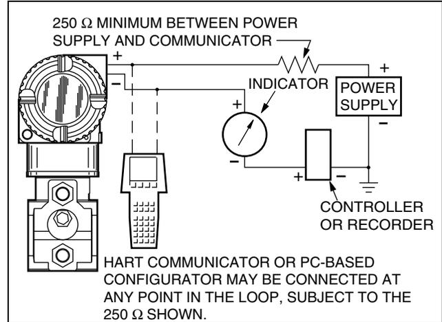
Figure 20. 4 to 20 mA Output Block Diagram
