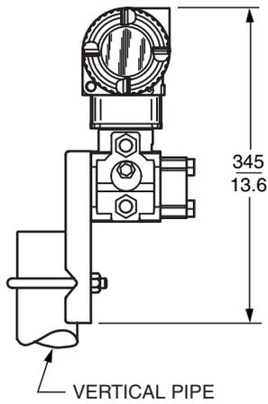
TRANSMITTER WITH LOW PROFILE STRUCTURE LP2
