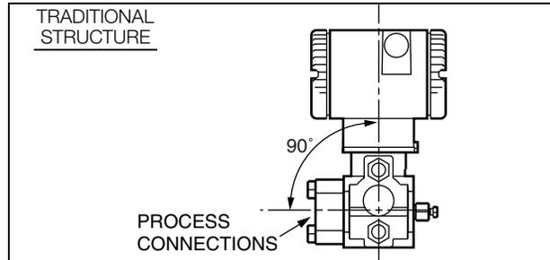
Figure 3. Vertical Mounting Showing Process Connections at 90 degrees
