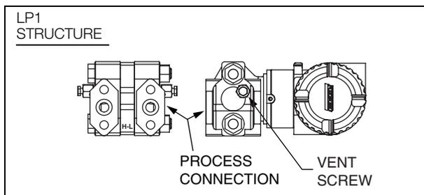
Figure 11. Horizontal Mounting with Vent Screw
