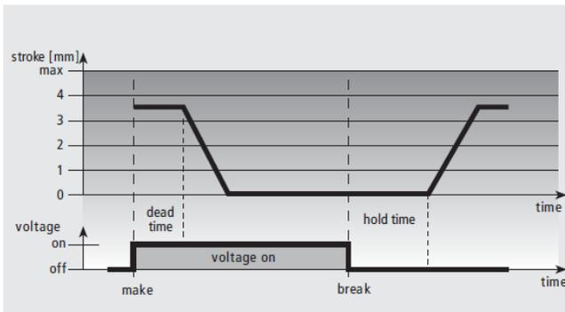
In case of the normally open version, the valve is closed evenly by the ram motion upon switching on the operating voltage and after expiry of the dead time.
