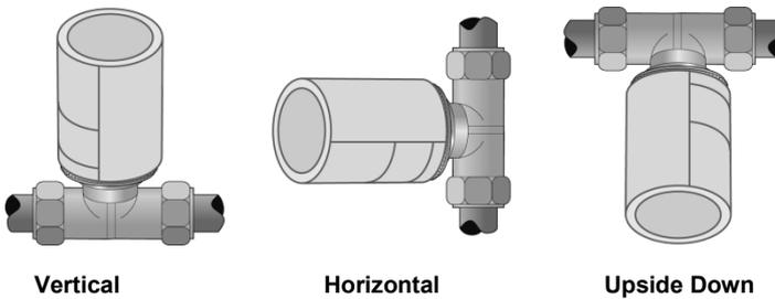
Preferred installation position of the OEM-Actuator is vertical or horizontal. An upside down position may reduce product life through special circumstances (e.g. contaminated water).
