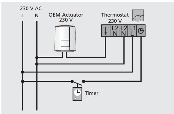
We recommend usage of the following lines for installing a 230 V system:
