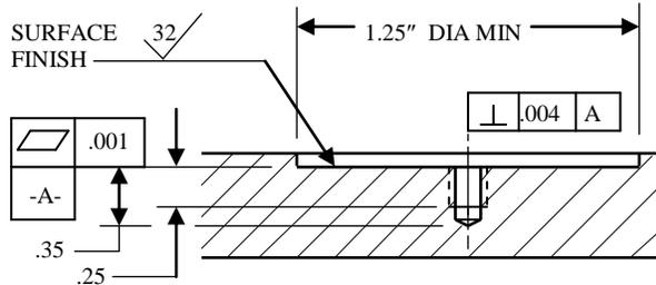
Before stud mounting the transmitter, a coupling fluid should be applied to the mating surfaces. The coupling fluid protects the mounting surface and optimizes the frequency response by increasing the coupling stiffness. Suggested coupling fluids are machine oil or vacuum grease. It is recommended that a thread adhesive such as Loctite 222 be used.
