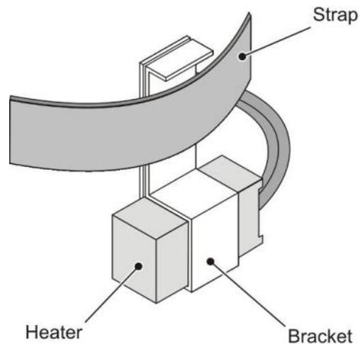
*Fig 19 Anti-Condensation Heater*
