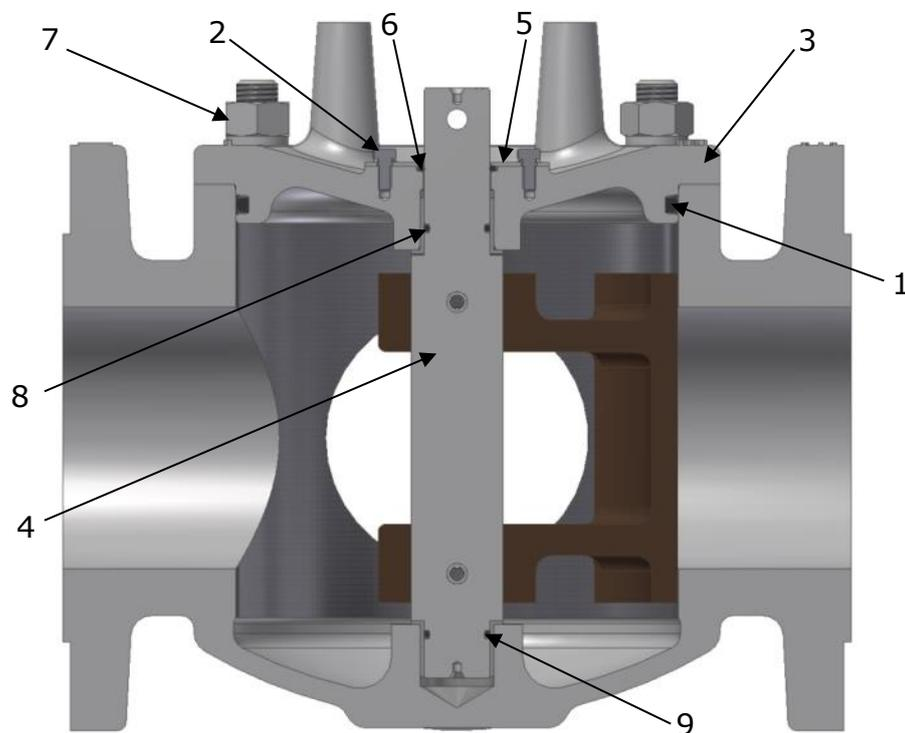
*Fig 4 Section View (04GGH illustrated)*
