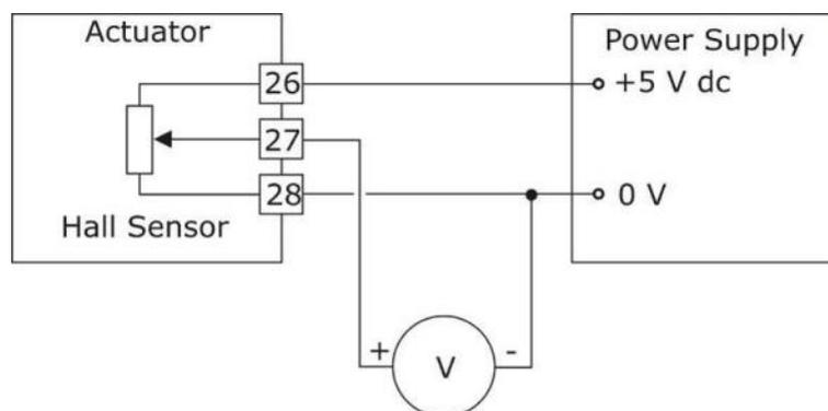
*Fig 18 Electrical Connections for Sensor Alignment*
