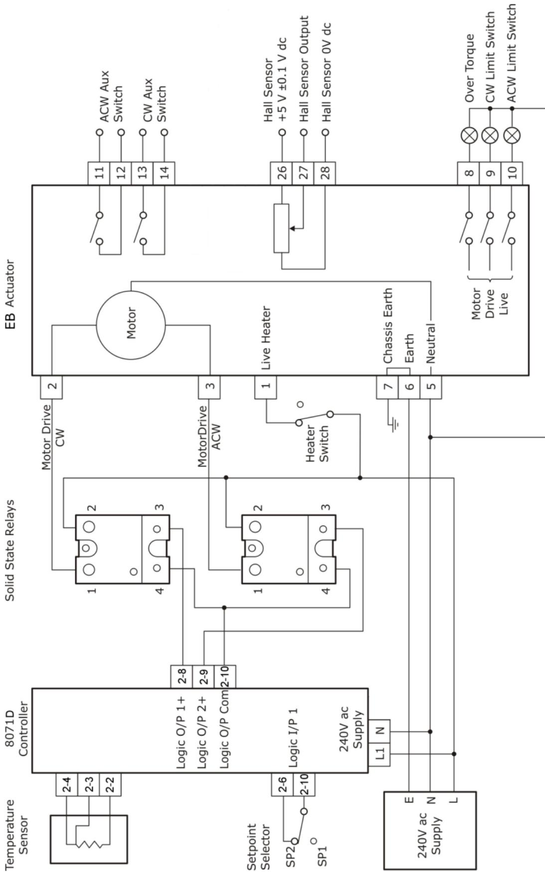
Fig 24 8071D controller with 2 solid state relays
