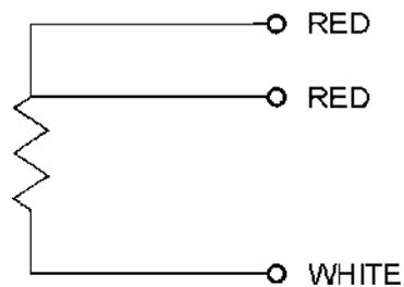
*Fig 22 Temperature Sensor Connections*
