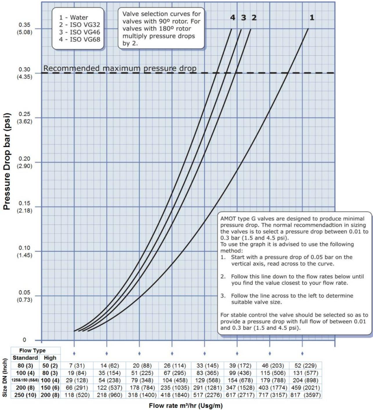
Fig 30 Valve Selection Curve
