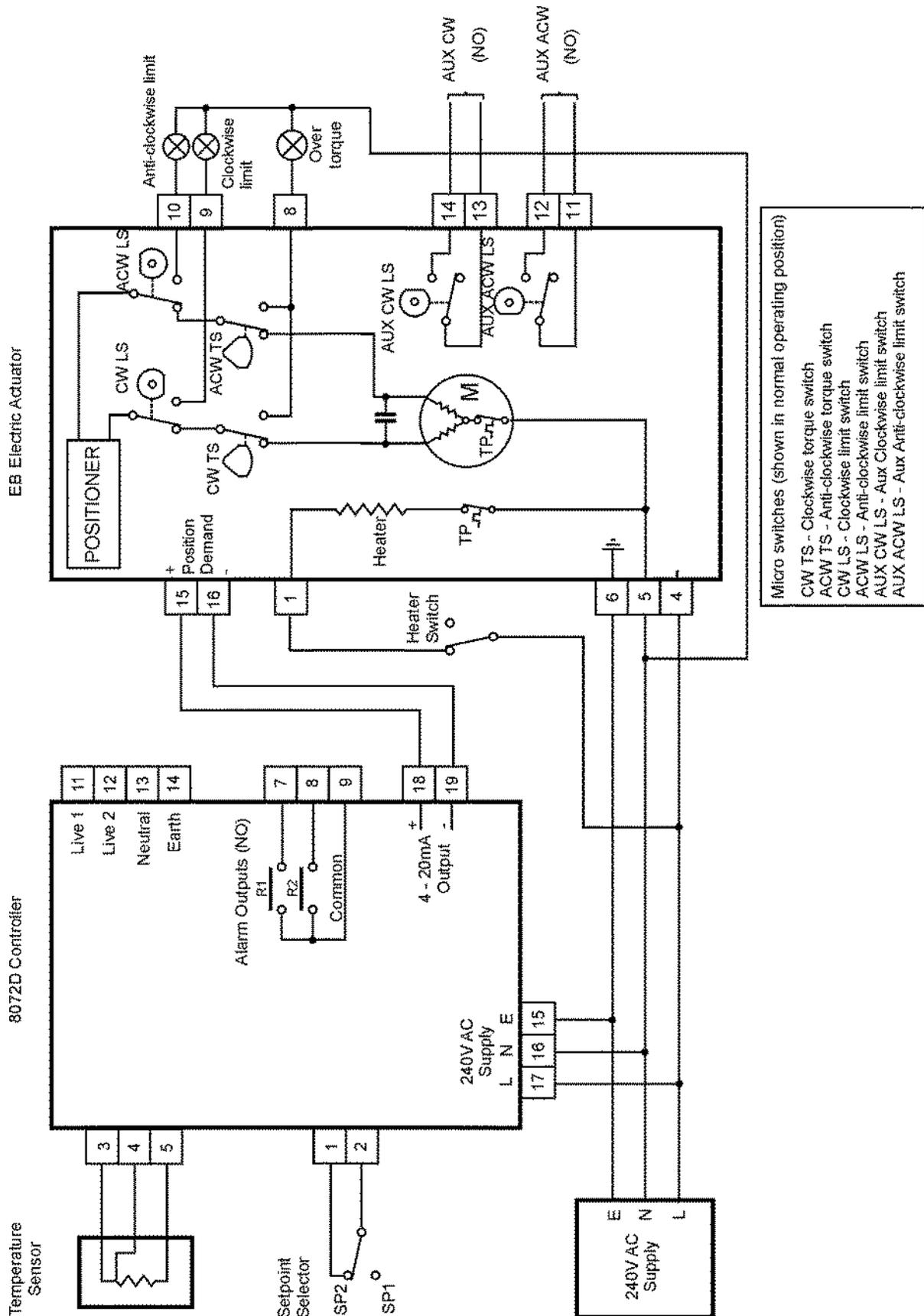
Fig 27 8072D controller (Actuator with Positioner)
