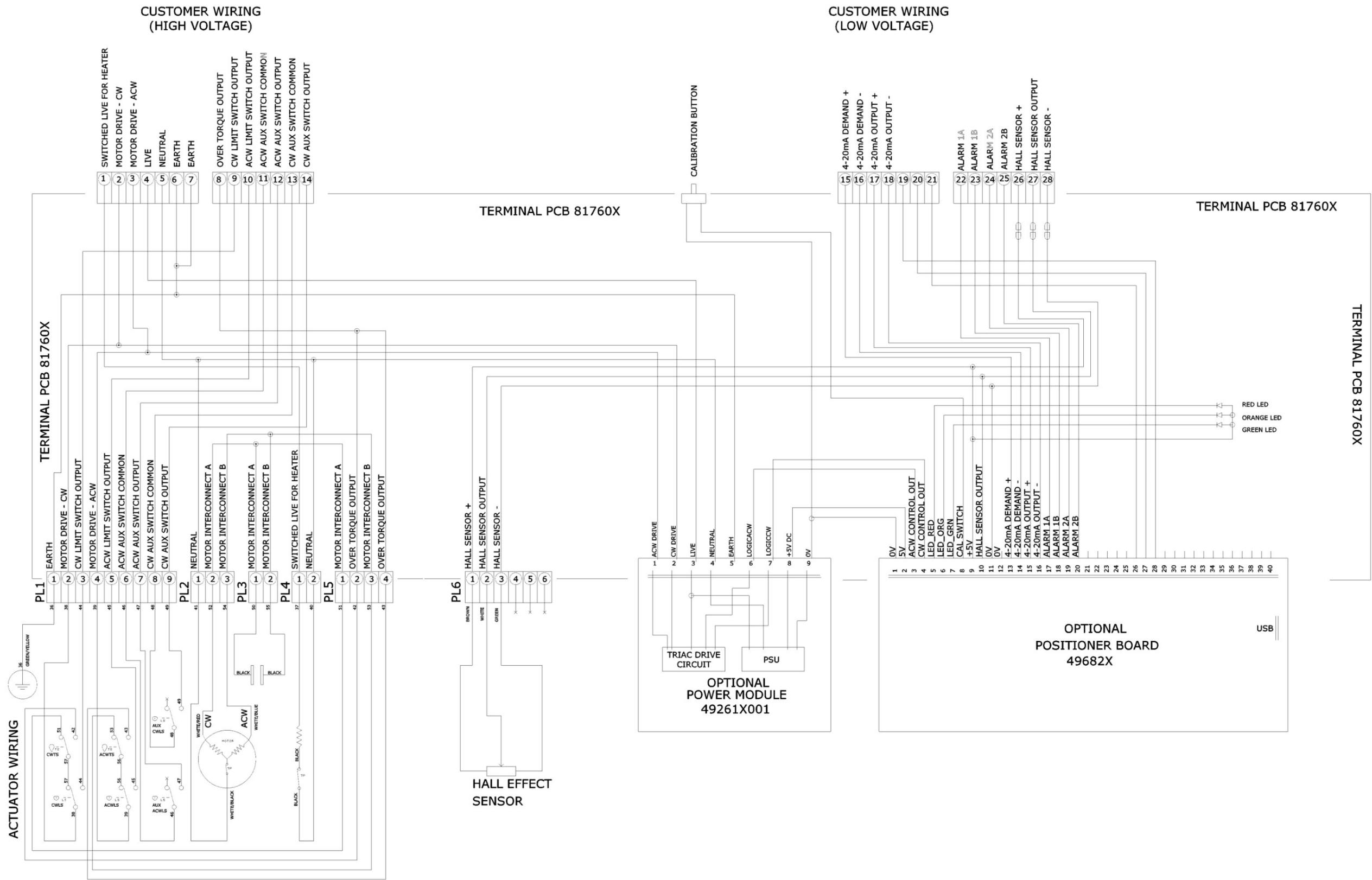
Fig 7 Wiring Diagram – EB Actuators
