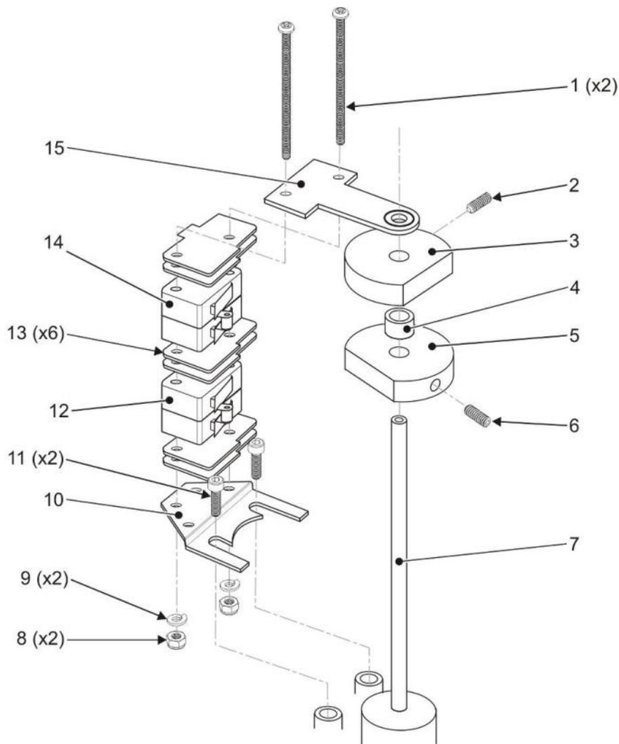
*Fig 16 Limit Switch Assembly and Cams*
