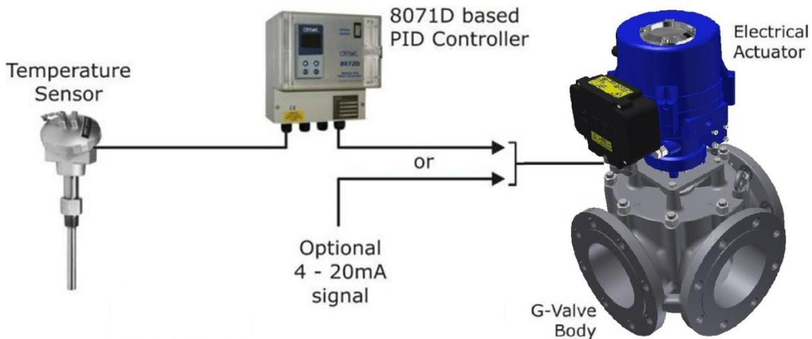
Fig 2 System Components
