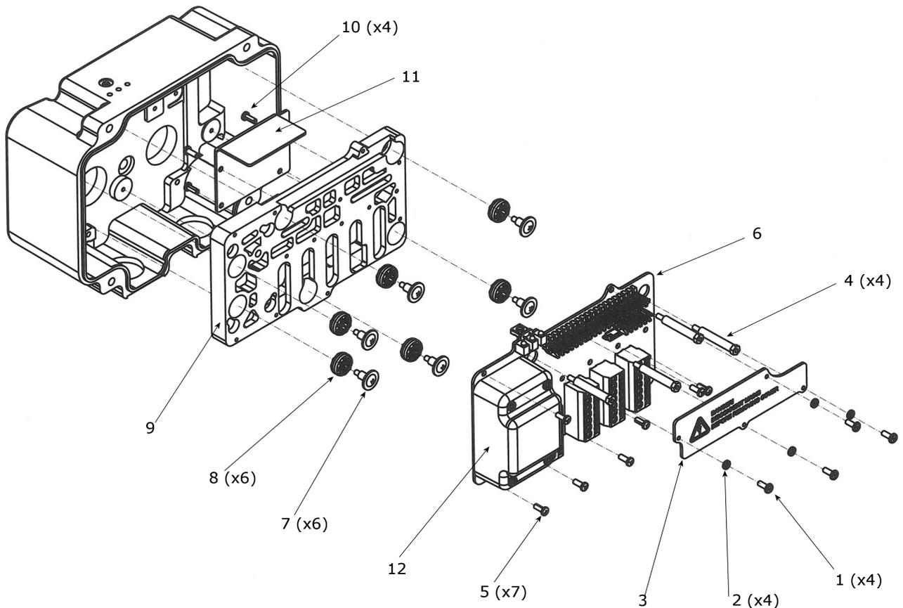
*Fig 20 Terminal Board*
