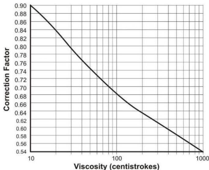
Fig 31 Viscosity Correction Graph
