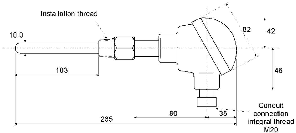
*Fig 21 Temperature Sensor*
