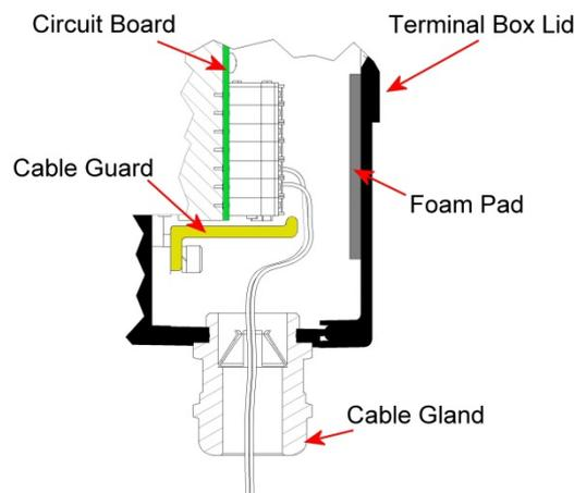
*Fig 10 Cable routing*
