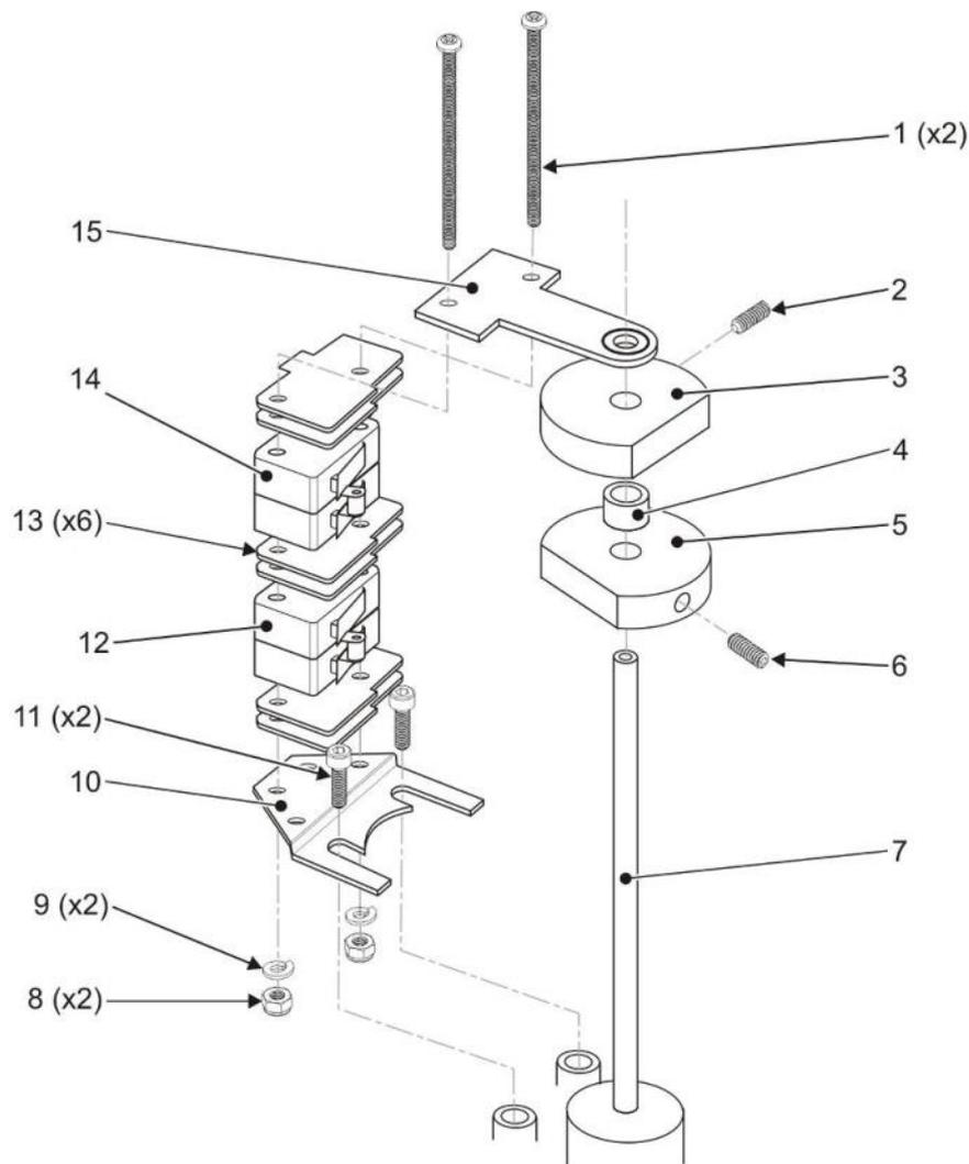
Fig 17 Limit Switch Adjustment
