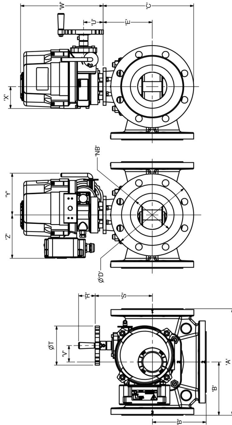
*Fig 32 Valve Dimensions*
