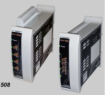
Series of galvanic isolators composed of independent cells designed for the 0..4..20mA current loop processing. Each input may be wired in active or passive mode, so it is able to measure a current provided by an active transmitter or to supply a 2-wire transmitter and measure the loop current.
