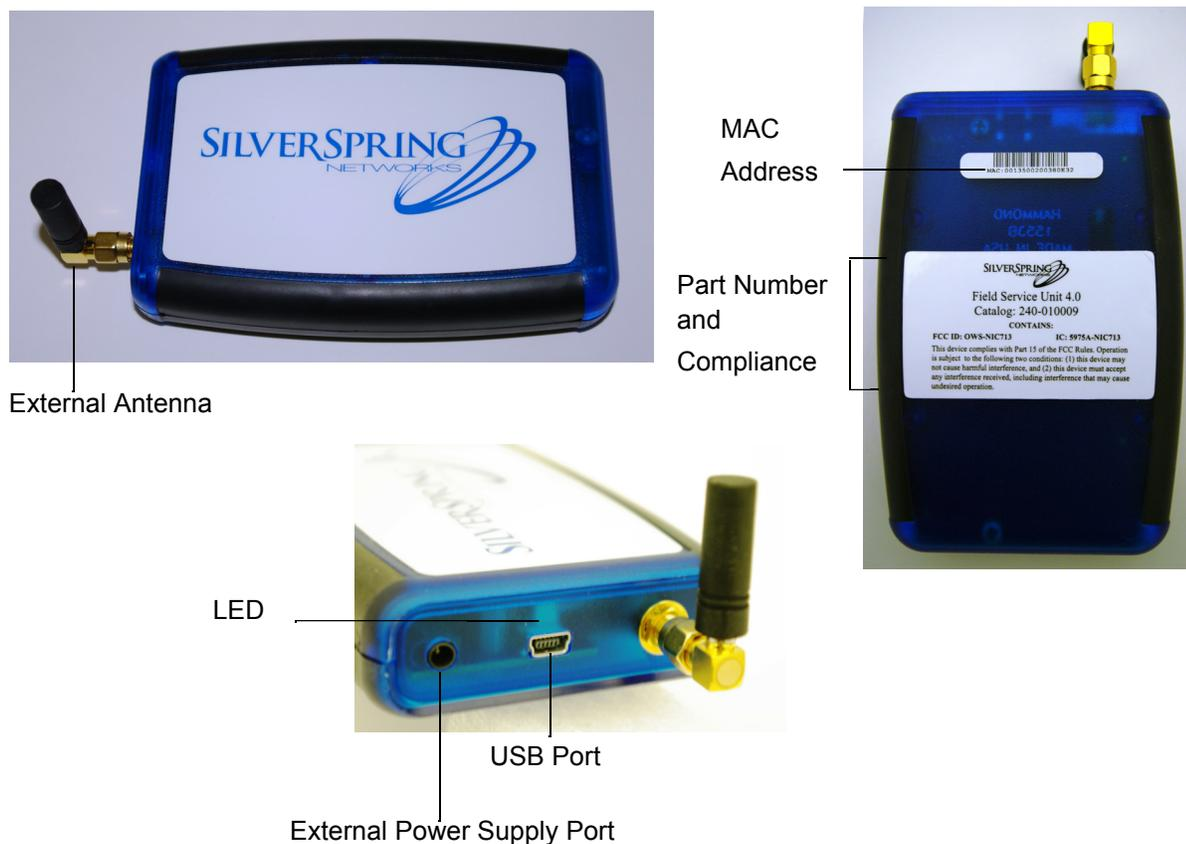
You can switch between the on-board antenna and external antenna using commands in Communications Tester field tool.
