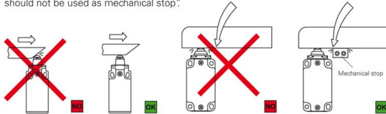
The actuator must not exceed the max. travel as indicated in the
