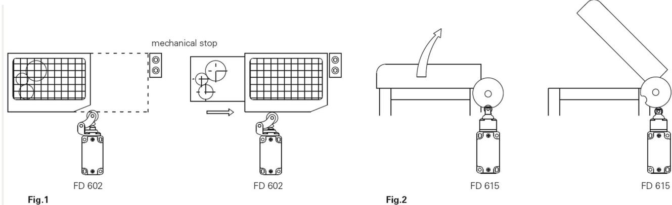
In the safety application with only one switch for each guard, the switches **should not be applied to activate by release** (fig. 3 and 4) **or through a non rigid connection** (i.e. by a spring).
