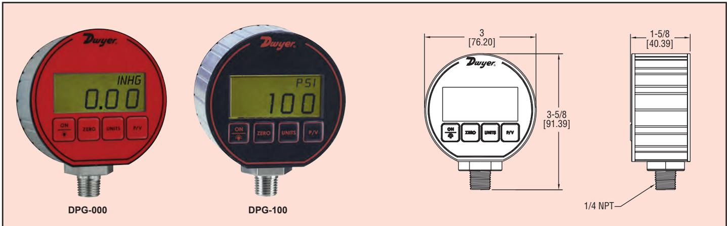
Replace your outdated analog gages with the new **Series DPG Digital Pressure Gage**. The Series DPG has a high ±0.25% or ±0.5% full-scale accuracy. The 4 digit digital display will reduce the potential for errors in readings by eliminating parallax error commonly produced with analog gages.
