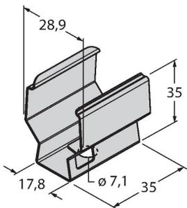
Snap bracket for mounting WLS28 work lights
