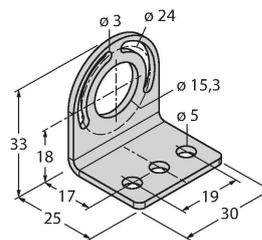
Mounting bracket, angled, metal, for WLS28 work lights, 5 mm drill holes, screw set included
