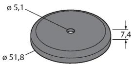
Magnetic mounting bracket for mounting on metallic surfaces, for mounting WLS28 work lights
