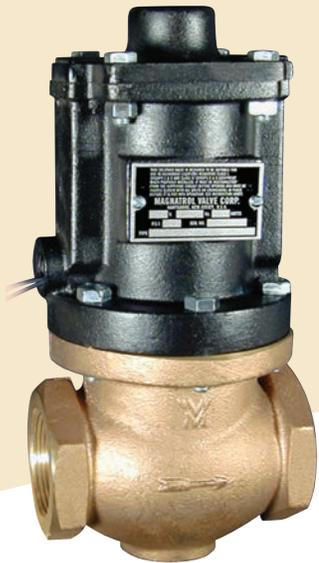
**OPERATION:** Valve opens when energized and closes when de-energized. When the coil is energized the pilot valve opens, relieving the pressure above the piston, which is then lifted from its seat by the plunger. Upon de-energizing the coil, a spring closes the pilot valve and opens a bleed passageway to permit pressure to build above the piston and seat it.
