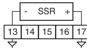
**Logic level 0:**  $V_{out} < 0.5$  VDC;
