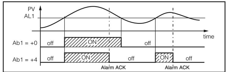
4. A “Relative alarm not active at set point change” is an alarm that masks the alarm condition after a set point change until process variable reaches the alarm threshold plus or minus hysteresis.
