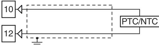
**Input circuit:** Current injection (25  $\mu$ A).
