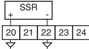
**Logic level 0:**  $V_{out} < 0.5 \text{ VDC}$ ;
