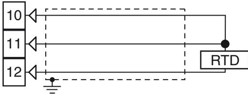
**Input circuit:** Current injection (135  $\mu$ A).
