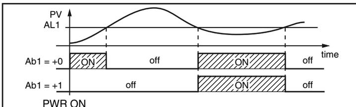
2. A “Latched alarm” (manual reset) is an alarm that remains active even if the conditions that generated the alarm no longer persist. Alarm reset can be done only by an external command (U button, digital inputs or serial link).
