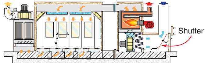
During the passivation and drying phases, the operator is out of the booth and the system closes the air shutter to recycle the internal air in order to reduce the power consumption.
