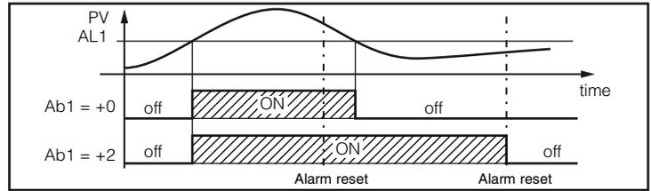
3. An “Acknowledgeable” alarm is an alarm that can be reset even if the conditions that generated the alarm are still present. Alarm acknowledge can be done only by an external command (U button, digital inputs or serial link).
