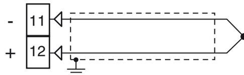
**External resistance:** 100Ω max., maximum error 0.5% of span.
