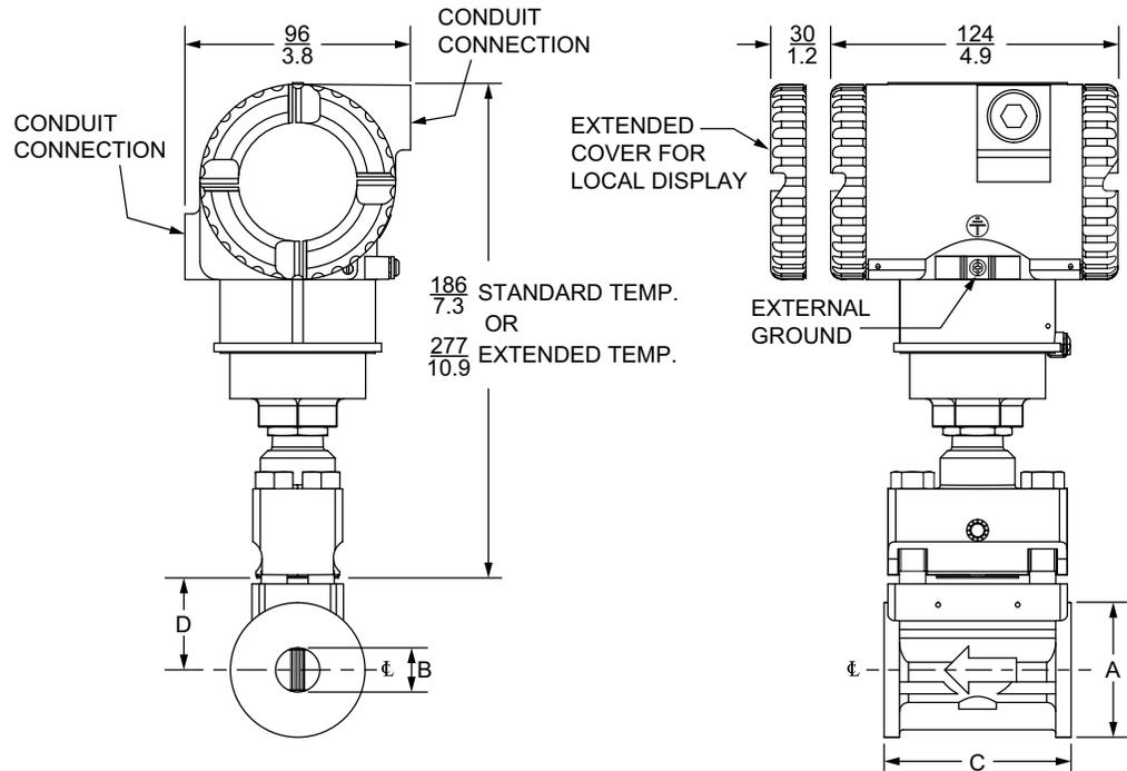
**Figure 7 - Wafer Body Flowmeter with Junction Box**
