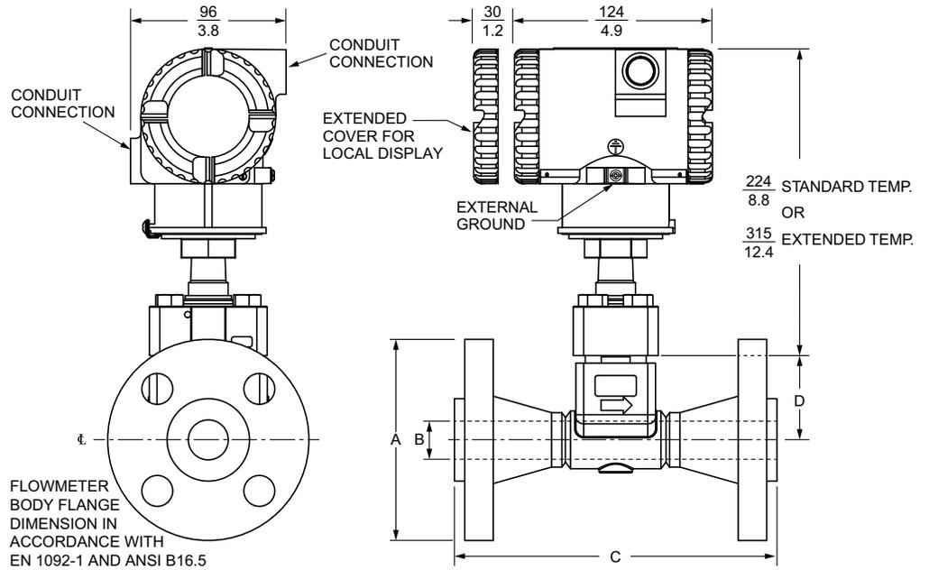
**Figure 4 - Flanged Body Flowmeter with Junction Box**
