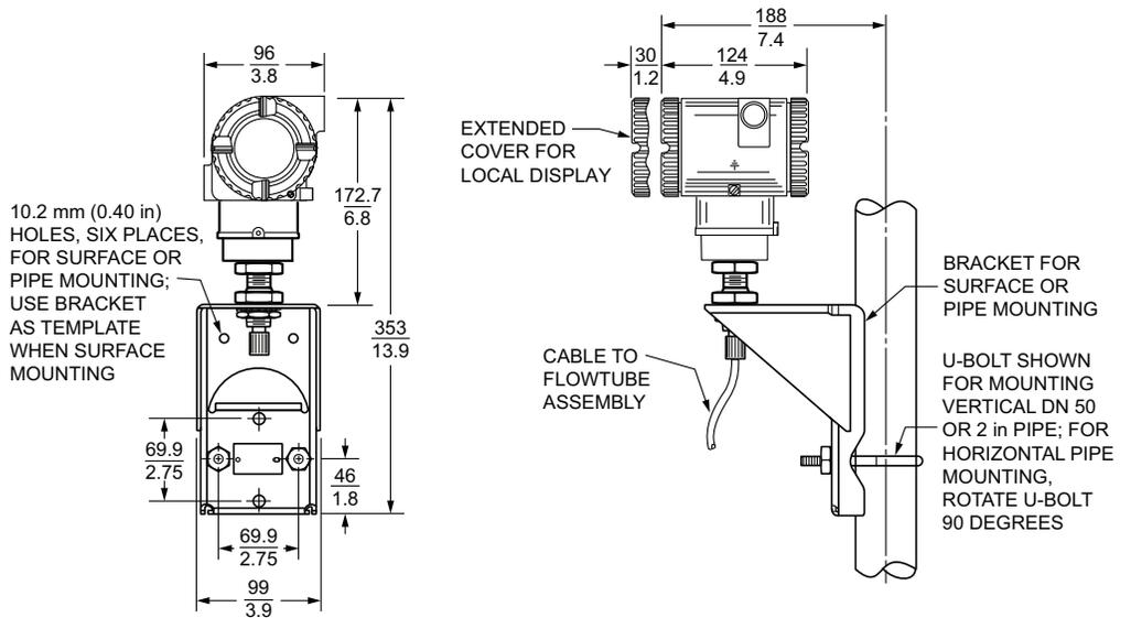
**NOTE:** WHEN THE BRACKET IS USED FOR WALL MOUNTING, REPLACE THE U-BOLT WITH TWO OR FOUR 0.375 in BOLTS LONG ENOUGH TO PASS THROUGH THE BRACKET AND SURFACE.
