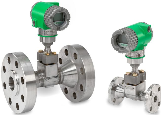
When configured with Multivariable selection T, the Model 84C Vortex flowmeter provides a process temperature measurement using the optional integral temperature sensor. With calculations based on ASME steam tables<sup>3</sup>, the Model 84C is an excellent solution for the mass flow metering of saturated steam.
