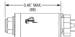
Fixed Plug to DIN 43650 Mating Connector Supplied
