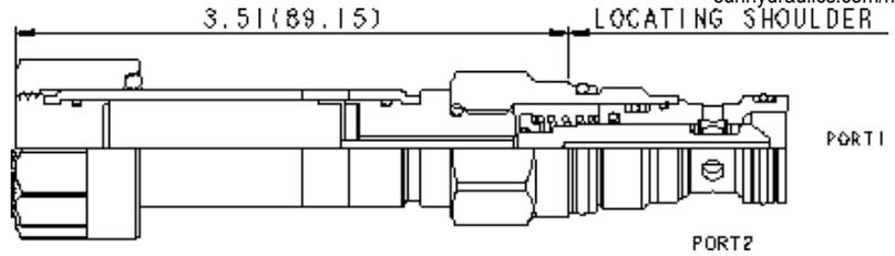
This solenoid-operated 2-way, 2-position cartridge is a direct-acting, poppet-style directional valve. The valve is available in either a normally open or normally closed configuration. Due to the poppet style construction, this valve has extremely low leakage.
