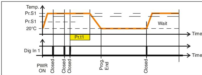
When a new panel is detected before the end of the first soak time, the program restarts and the set point remains equal to Pr.S1.
