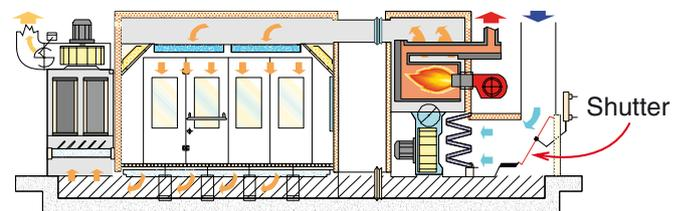
During the passivation and drying phases, the operator is out of the booth and the system closes the air shutter to recycle the internal air in order to reduce the power consumption.
