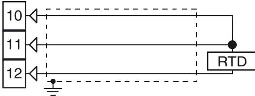
**Input circuit:** Current injection (135  $\mu$ A).
