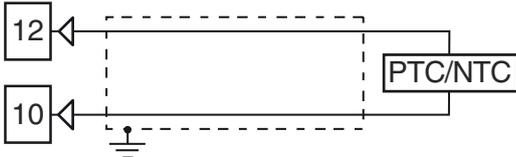
**Input circuit:** Current injection (25  $\mu$ A).
