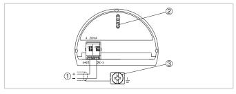
Electronics and terminal compartment, single chamber housing
