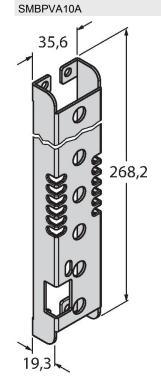
3062447 Mounting bracket, for PVA225, coldrolled steel, cut-out for DIP switch block, protection for light
