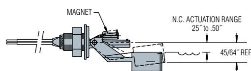
The LS-7 Type 12 is ideal for use on food warmers, hot water heaters, steam cookers, small boilers or wherever water evaporation occurs. The switch is used effectively for either high fluid level alarms or water make up systems. The units are made of Noryl®, which carries NSF approval for use in potable water, and are supplied with FDA-approved Buna gaskets.
