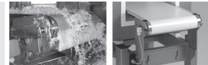
Friction drive belts are driven via the friction between drum motor and conveyor belt. The drum motor is normally crowned to prevent belt wander. The belt must be tensioned in order to transfer the torque from the drum motor. The top surface of the belt can be flat, plain or have a ribbed, grooved or diamond pattern.
