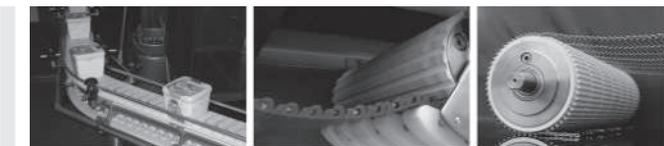
Modular plastic belts, solid homogeneous belts, steel mesh or wire belts are positively driven, i.e., with no belt tension. Since the belt has hardly any direct contact with the drum shell, the heat
