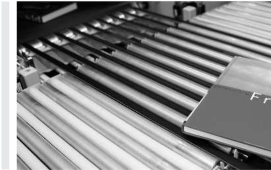
All Interroll Drum Motors excel with relatively low noise development and vibrations. The performance levels are not specified or guaranteed in this catalog because they can vary depending on the type of motor, number of poles, speed and application. For specific low-noise applications, please contact your Interroll customer consultant.
