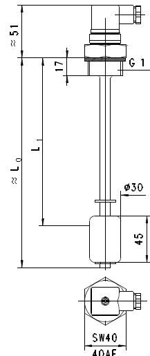
Details of float location L<sub>1</sub> mm for density 1 g/cm<sup>3</sup>
