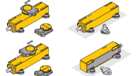
Extensive mounting accessories provide various options for installation.
