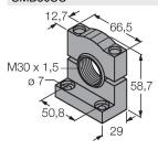
Mounting bracket, PBT black, for sensors with 30 mm thread, rotatable
