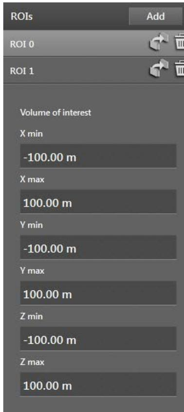
An ROI is set up via the x, y and z values in the world coordinate system. The volume of interest within the coordinate axes is used for the ROI.
