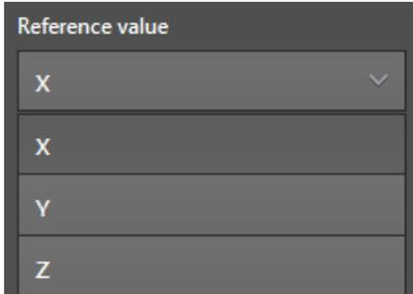
The "reference value" defines which output of the ROI groups is used as a basis for the colouring of the overlay. The following reference values can be selected:
