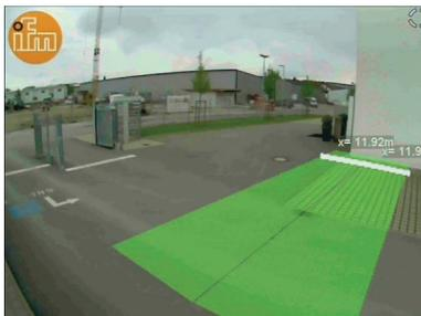
In the figure on the left, the provision of 2 ROI groups is visualised as a coloured overlay on the floor and the X values as a text.
