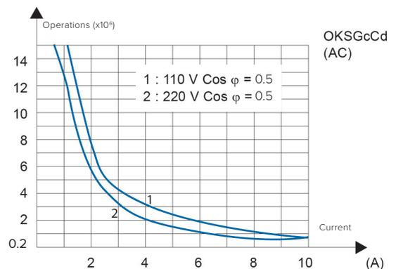
(I) Switching frequency 1,200 operations/hour, 50% cycle.
