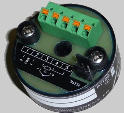
The CNL40ig is a universal smart in-head mounting temperature sensor transmitters. Cover all temperature measurement (RTD and thermocouples) in all range with an unique device. The CNL40igH integrate the HART communication protocol, FDT compliant and it is available with SIL2 conformity according to IEC 61508 standard.
