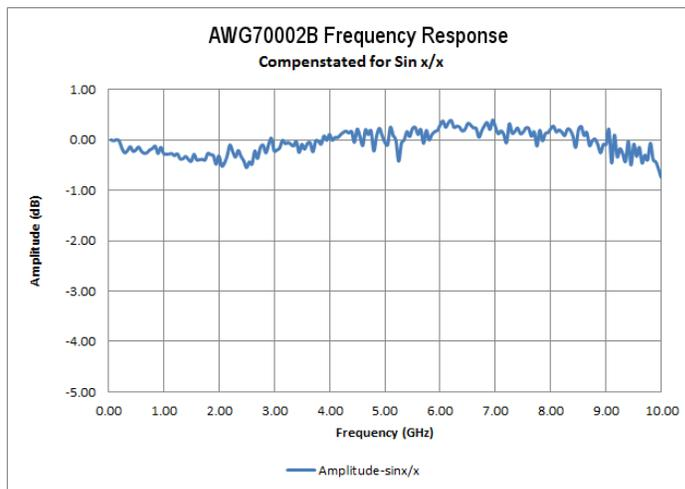
AWG70002B measured frequency response and ideal  $\text{Sin}(x)/x$  response at 25 GS/s.
