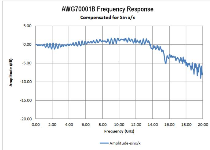
AWG70001B measured frequency response and ideal  $\text{Sin}(x)/x$  response at 50 GS/s.
