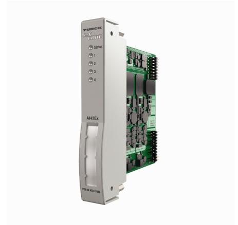
The analog input module AI43Ex is used for the connection of potentiometers in 3 or 4-wire technology. If 3-wire potentiometers are used, the terminals at the module rack have to be bridged. Resistance measurements, i.e. the evaluation of potentiometers with a 2-wire connection, is not possible.
