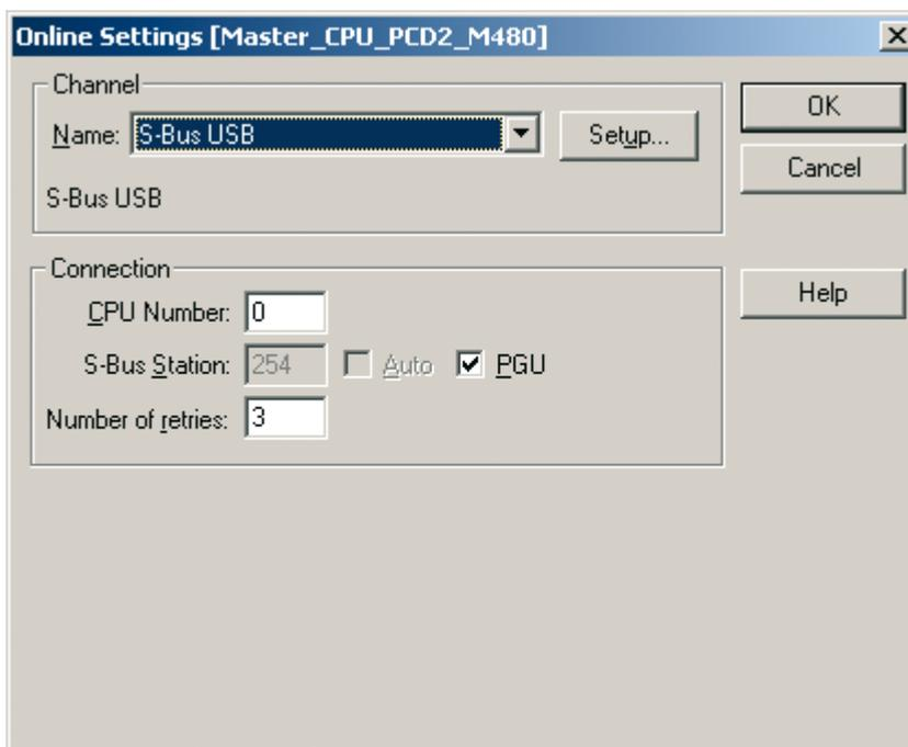
Activating the PGU option ensures that the PCD connected directly to the PC can be reached, regardless of the S-Bus address that has been configured.
