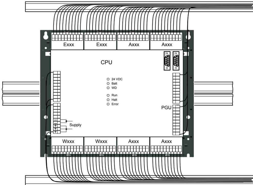
The cables to the terminals on the motherboard are run through the two side channels from the bottom or from the top.
