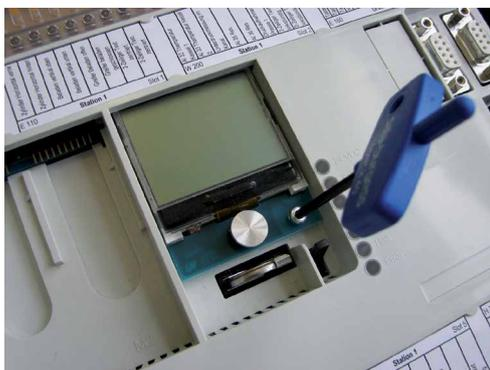
Insert the display into the aperture and push up to the stop. Fix with the screw provided (3 x 6 Torx plus).
