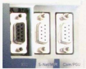
Push out pre-pressed aperture for the D-Sub socket and replace upper part of housing, section 3.5.4
