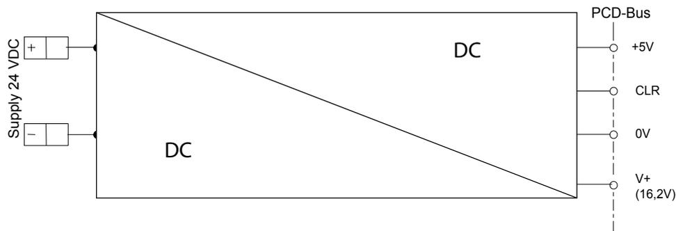
The PCD2.C2000/C1000 module holders provide the following internal supply currents to the modules plugged in or connected to them:
