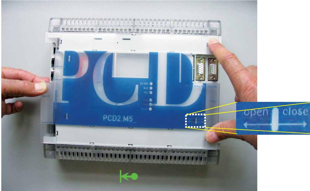
After removing the cover, the plug boards for flash cards, the lithium battery, the run/halt switch etc. are freely accessible.
