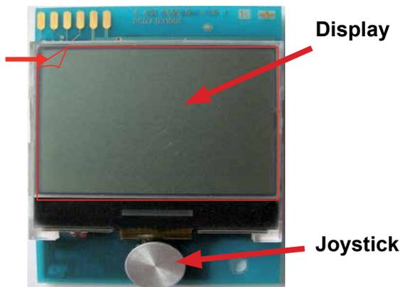
Remove the transparent protective film from the display
