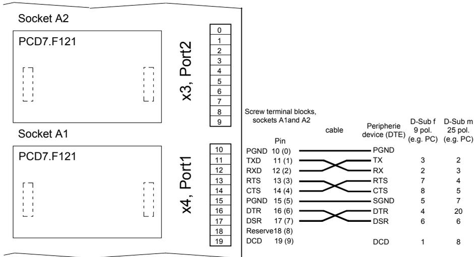
**RS-232 interface, for external modem (DCE)**
