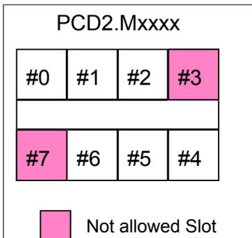
Two modem modules cannot be mounted side-by-side.
