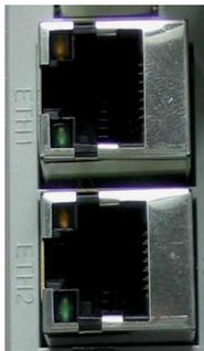
For these Ethernet connections, a new 10/100 Mbits switch is used, which switches automatically between the two speeds. Both sockets can be used independently of each other.
