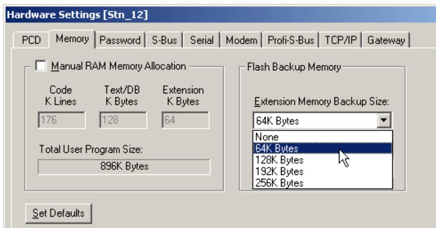
On the Memory tab, the Extension Memory Backup Size can be set. This memory size represents the memory space for the "Copy program to flash" function. On the left-hand side, the currently available memory space for the user program is displayed.
