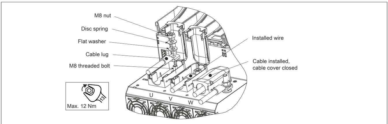
Figure 7: Motor connections U, V, W - Cable installation
