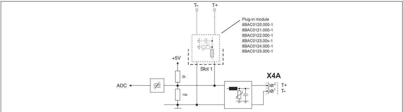
Figure 12: Temperature sensor
