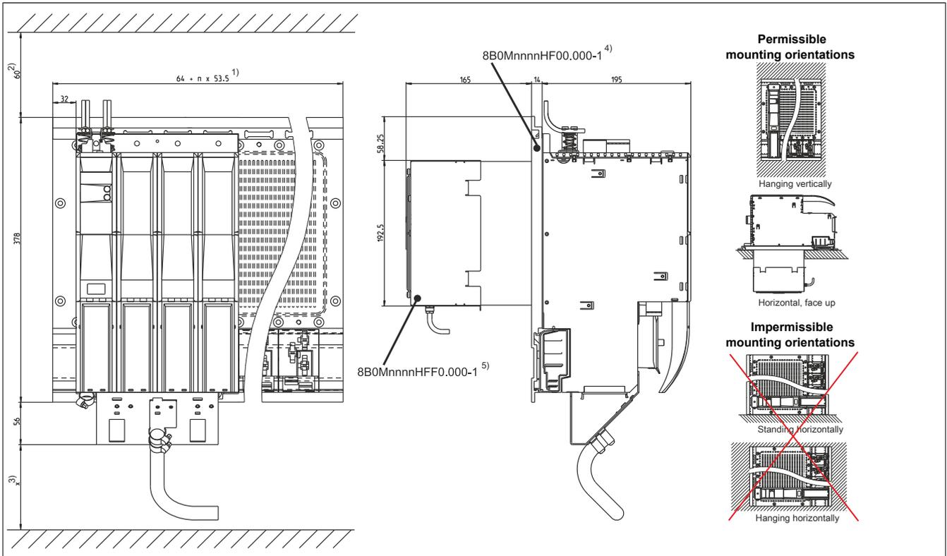
Figure 5: Pass-through mounting - Dimension diagram and installation dimensions
