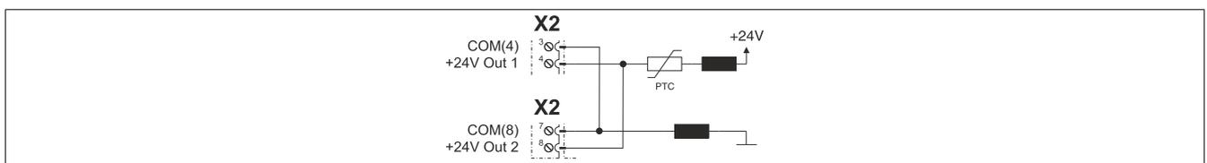
Figure 10: 24 VDC out
