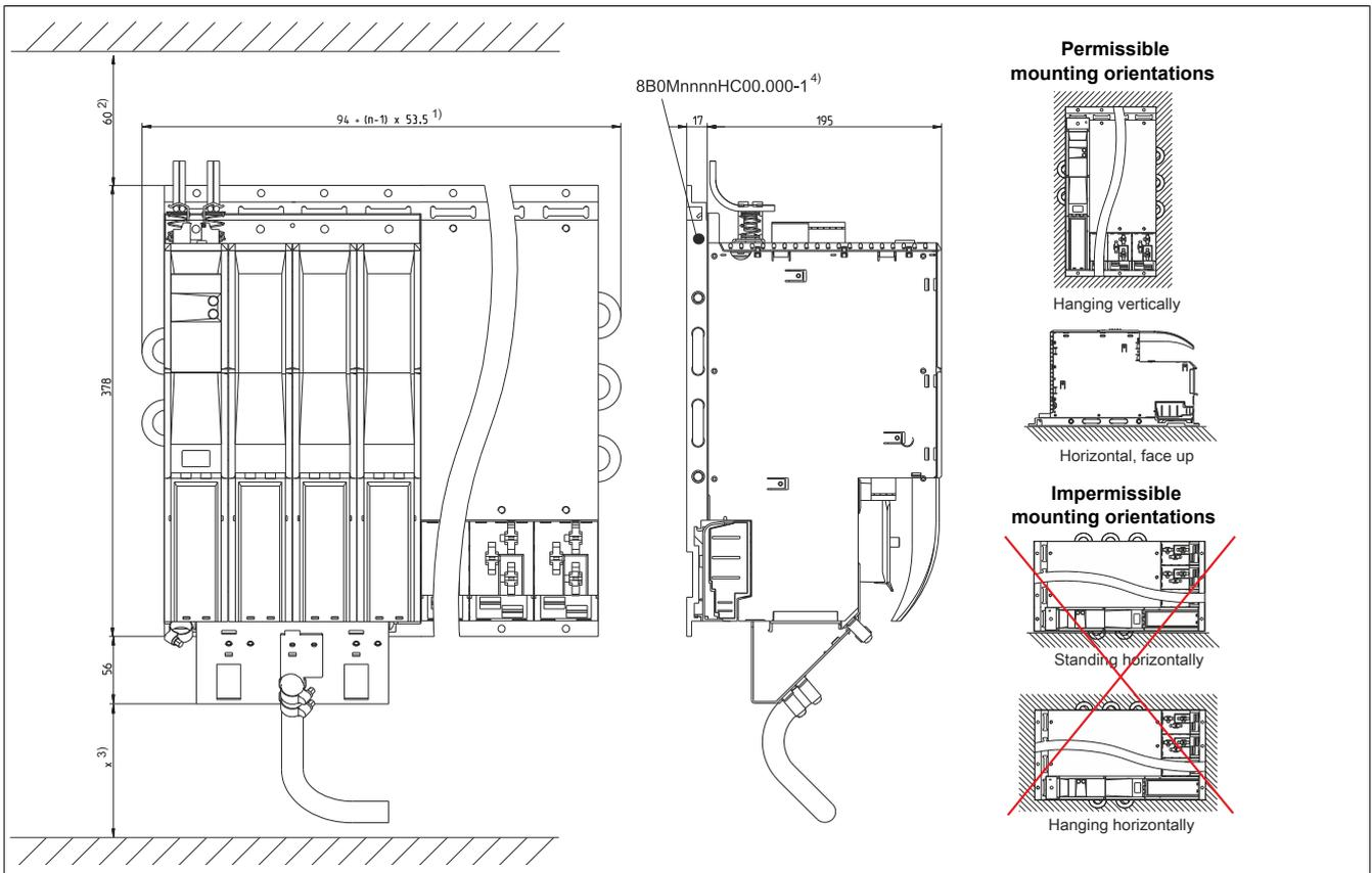
Figure 4: Cold plate - Dimension diagram and installation dimensions
