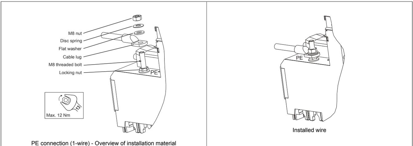
Table 18: PE connection (1-wire) - Cable installation
