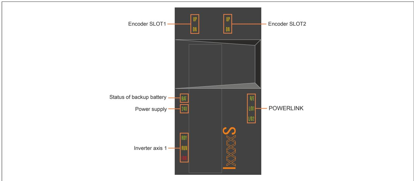
Figure 3: 8BVI inverter modules (1-axis modules) - Status indicator groups
