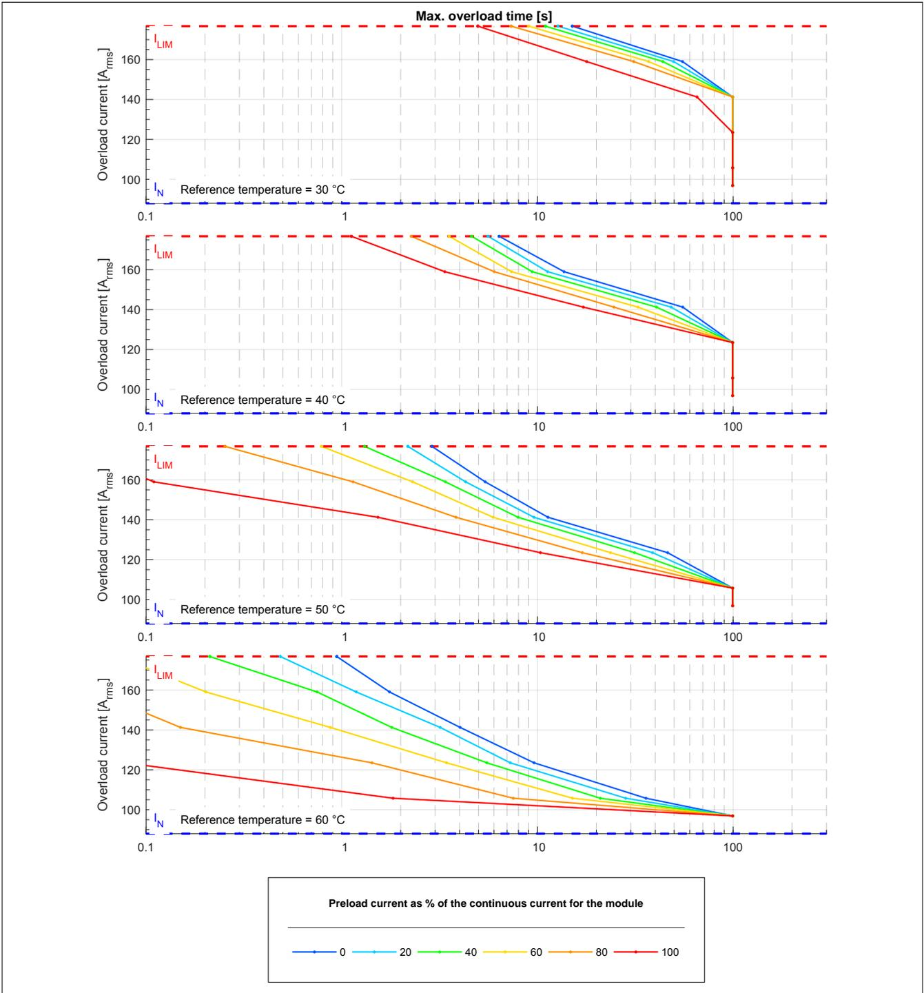
Figure 1: 8BVI0880HCSx.008-1 - Overload characteristics, overload response - WARNING
