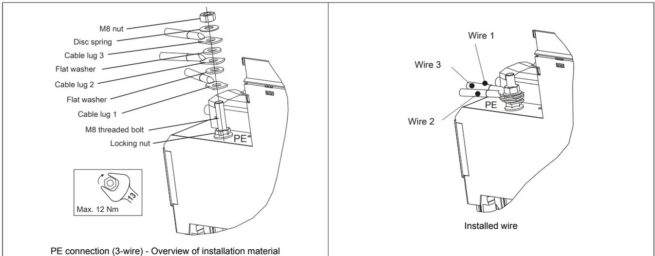
Table 19: PE connection (3-wire) - Cable installation
