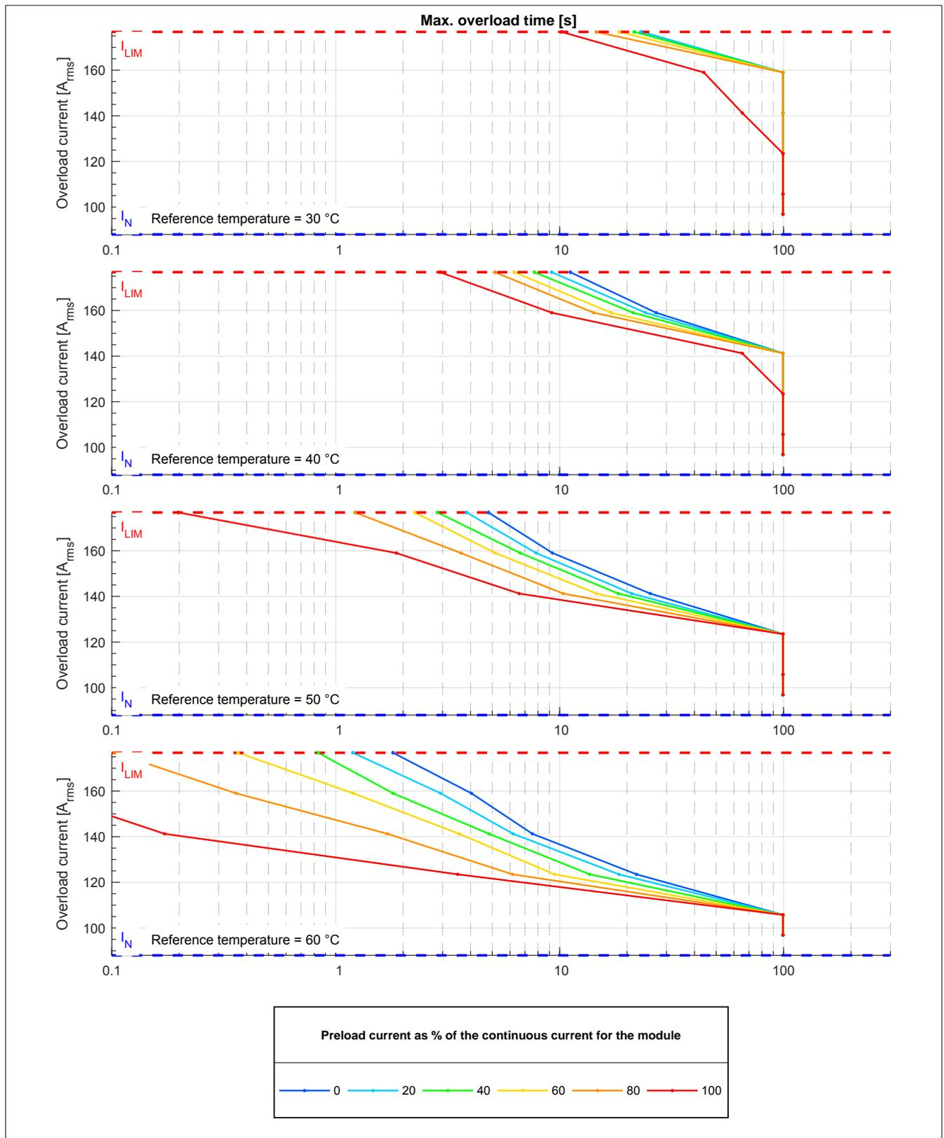
Figure 2: Overload characteristics of 8BVI0880HCSx.008-1, overload response - ERROR+STOP
