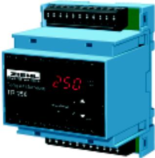
The Pt 100 thermostat TR 250 is a temperature controller and monitors up to 3 sensors Pt 100, Pt 1000, KTY 83 KTY 84 or thermistors (PTC) at the same time. Different types of sensors, e.g. Pt 100 and PTC can be monitored simultaneously. The unit is especially suitable for monitoring motors, generators and transformers. An other application is the use as a 2- or 3-step-controller with additional monitoring of over- or under-temperature or monitoring of differences in temperatures of 2 sensors.
