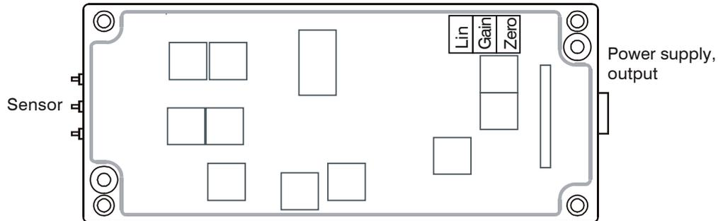
*Fig. 16 Potentiometers on the demodulator board*
